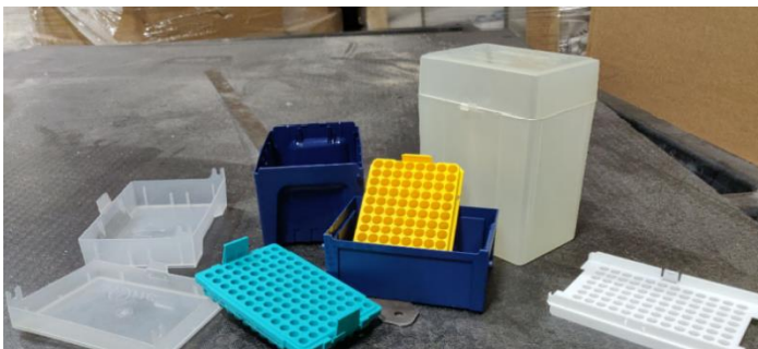
Figure 20. Pipette tip boxes of made from (PP), they must be empty and clean to be able to be recycled. (© L&T Ympäristöpalvelut Oy).
