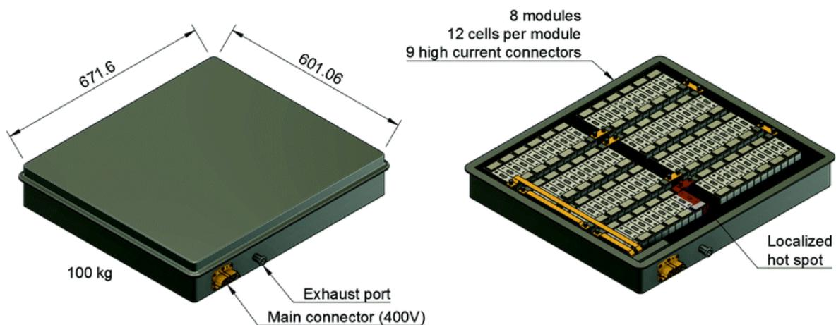
Figure 1. Hypothetical PHEV battery-pack. (Golubkov, A.W & Planteu, R & Krohn, P & Rasch, B & Brunnstener, B & Thaler, A & Hacker, V. 2018)
