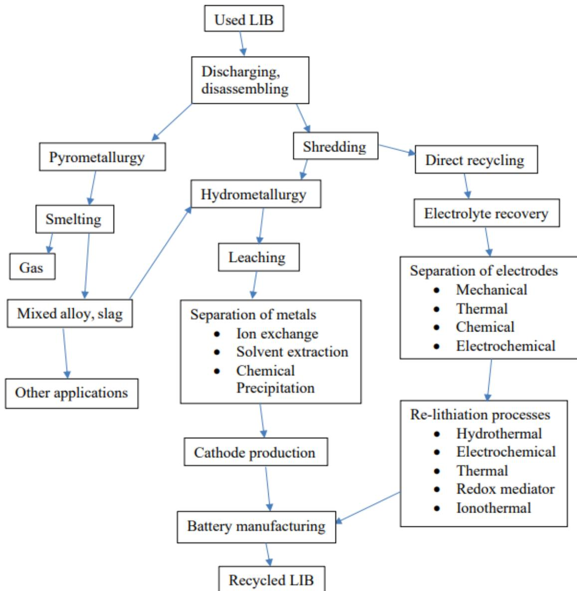
Figure 9. Main LIB recycling processes step by step.
