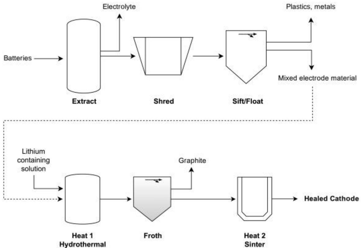
Figure 8. Scalable Cathode-healing™ process. (Sloopa, 2020)
