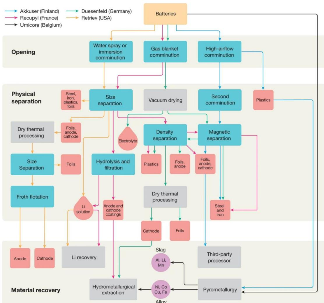
Figure 9. Different recycling systems in Europe and USA. (Harper, 2019)
