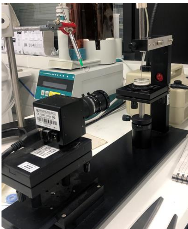
Figure 10. Sessile drop experiment setup.
