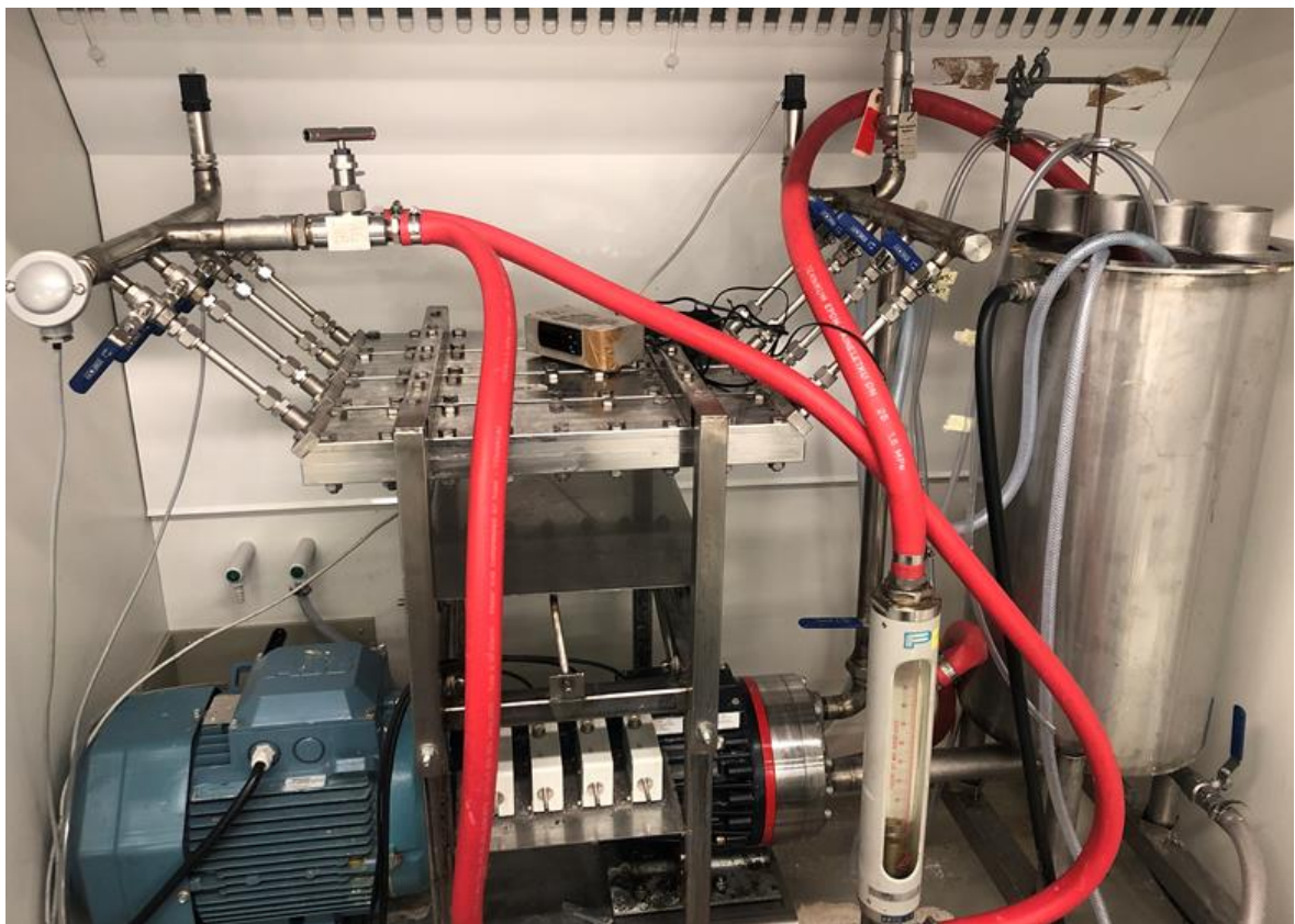
Figure 8. Cross-flow nanofiltration system with four parallel membrane modules.
