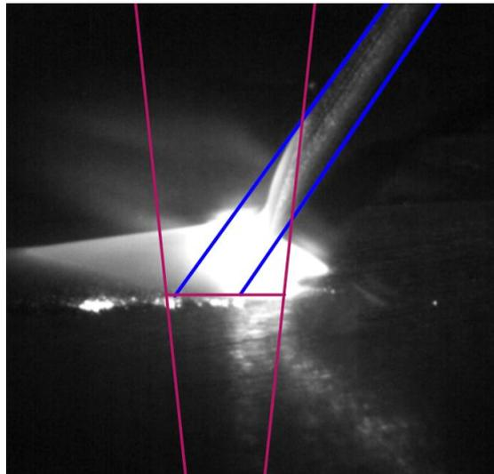
Figure 4. Position of the laser and wire drawn onto a monitoring image.
