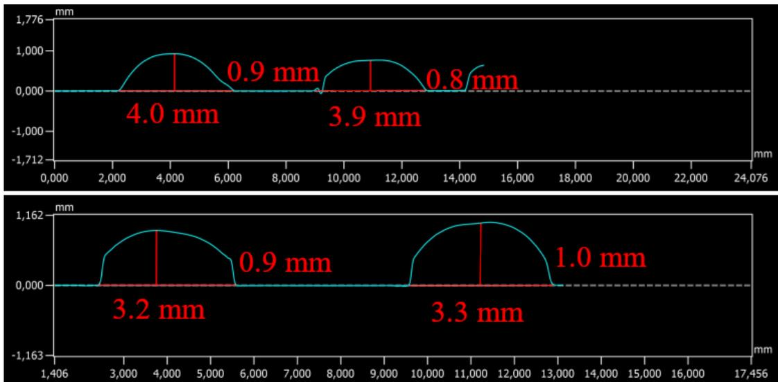
Figure 12. Heights and widths of the tracks. Top left: front feeding, top right: rear feeding, bottom left: side feeding away from the camera, and bottom right side feeding towards the camera.
