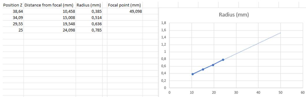
Figure 5. Laser spot radius calculation from PRIMES laser diagnostics software data.
