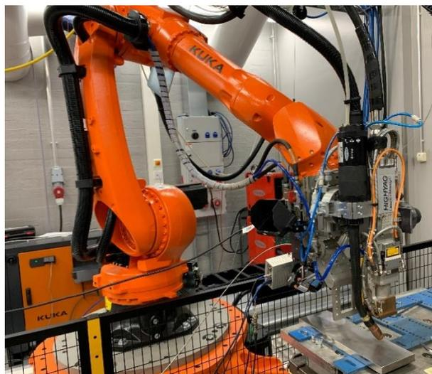
Figure 3. Image of the entire DED setup, with the deposition head connected to the KUKA robot.
