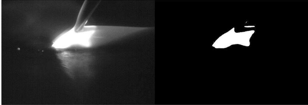
Figure 9. Rear feeding of filler wire (left). A binary image of the image on the left showing the melt pool (right).
