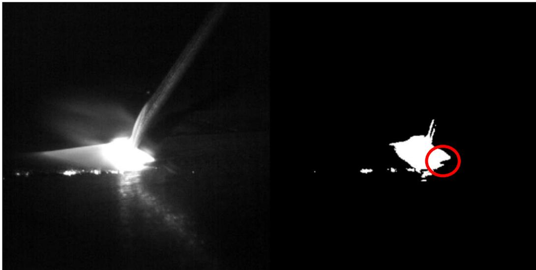
Figure 8. Image extracted from the monitoring system for front feeding of filler wire (left). A binary image of the image on the left, which shows the melt pool (right).
