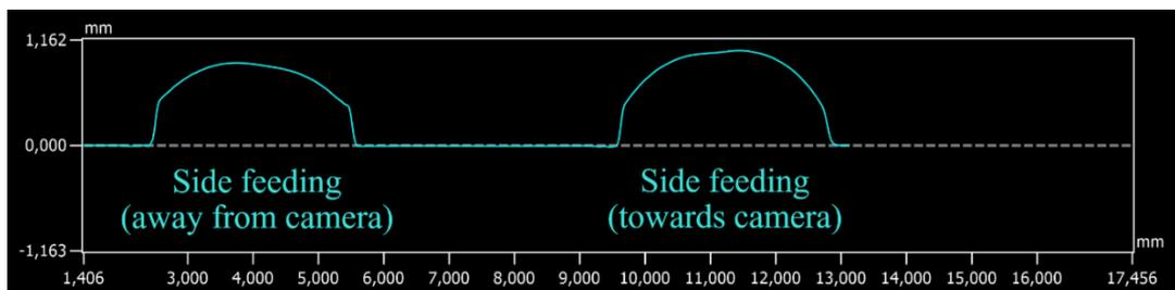
Figure 7. 3D measurement of the side feeding tracks
