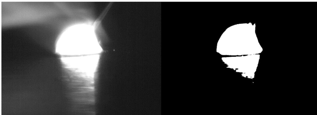
Figure 10. Side feeding of filler wire towards the camera (left). Binary image of the image on the left showing the melt pool (right).
