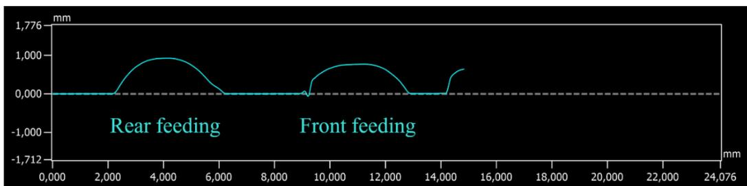
Figure 6. 3D measurement of the rear and front feeding tracks
