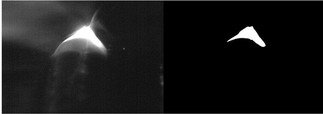
Figure 11. Side feeding of filler wire away from the camera (left). Binary image of the image on the left showing the melt pool (right).
