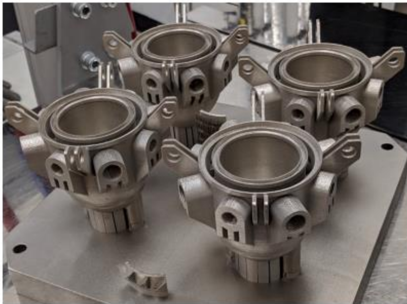
Figure 6. Swirlers used in the study after printing. (Adamou et al., 2021)
