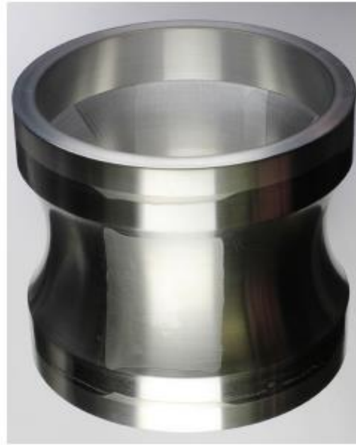
Figure 9. Rotor part for an electric motor made from NdFeB-Al composite and pure iron. (Lamarre, Bernier, 2019)
