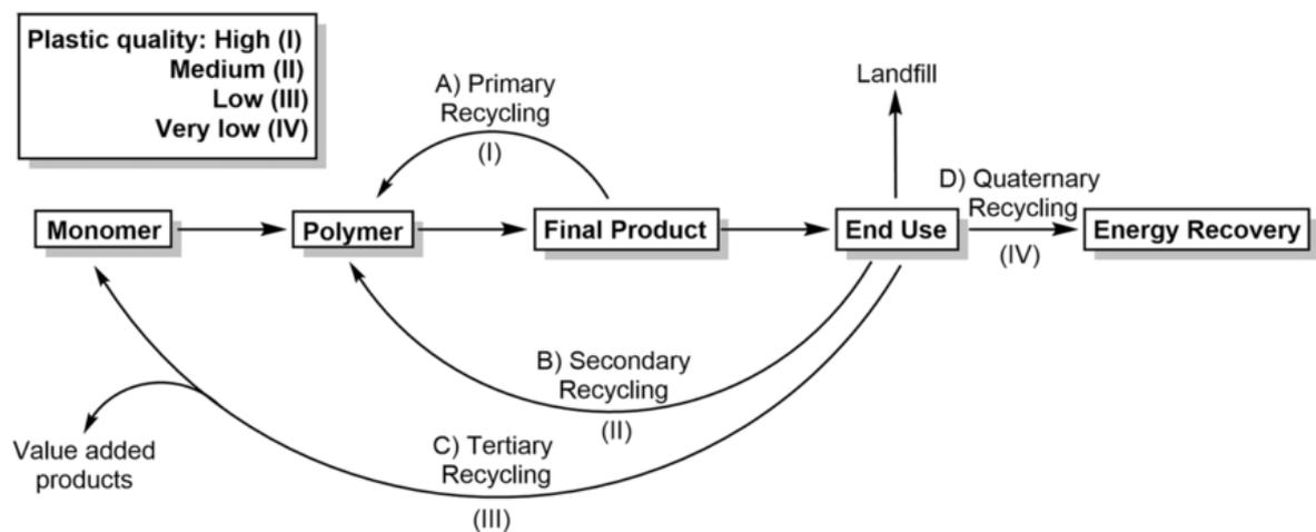
Figure 8 Plastic waste treatment options associated to necessary plastic quality. (Lamberti et al., 2020, 2.)
