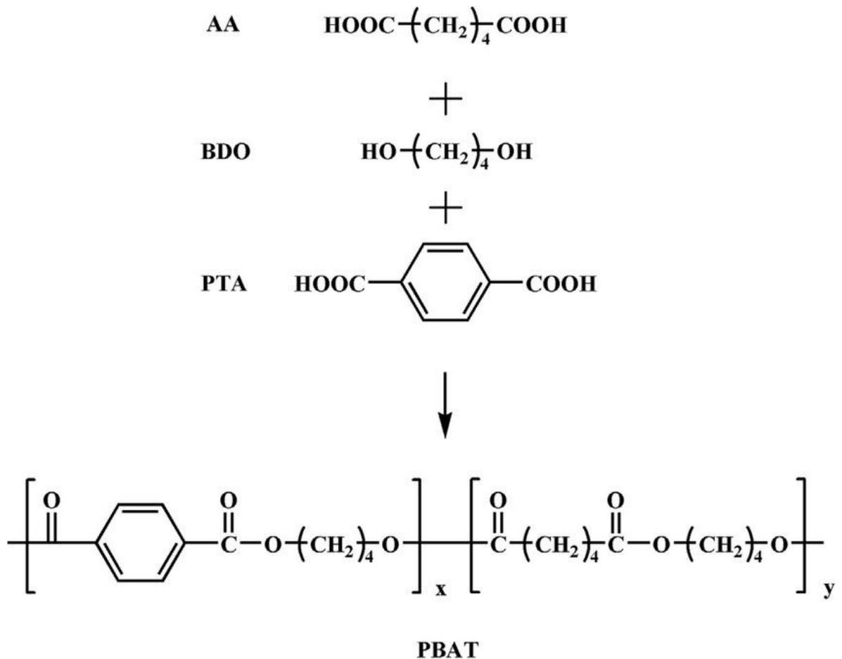
Figure 5 Reactants and schematic diagram of PBAT synthesis (Jian et al., 2020, 2).
