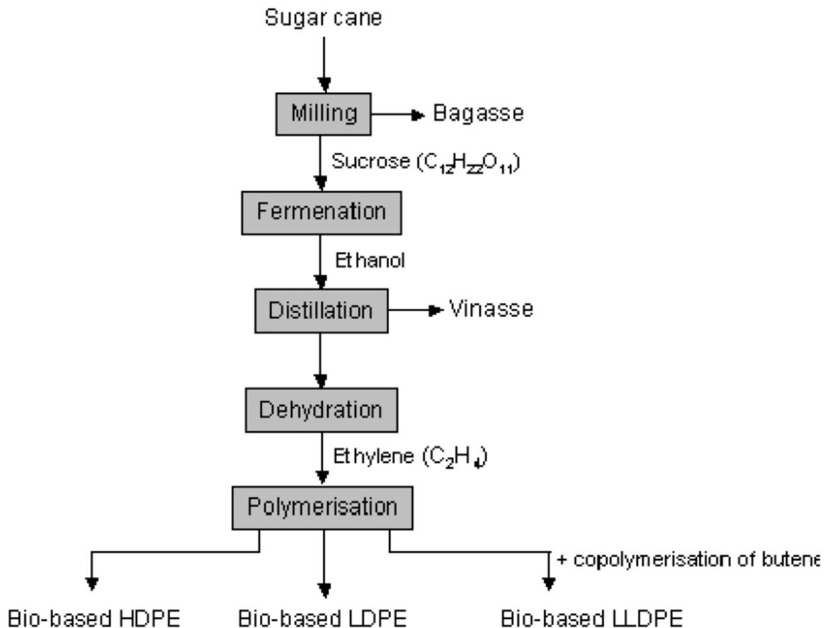
Figure 4 Production route of different biobased PE plastics (Shen et al., 2009, 133).
