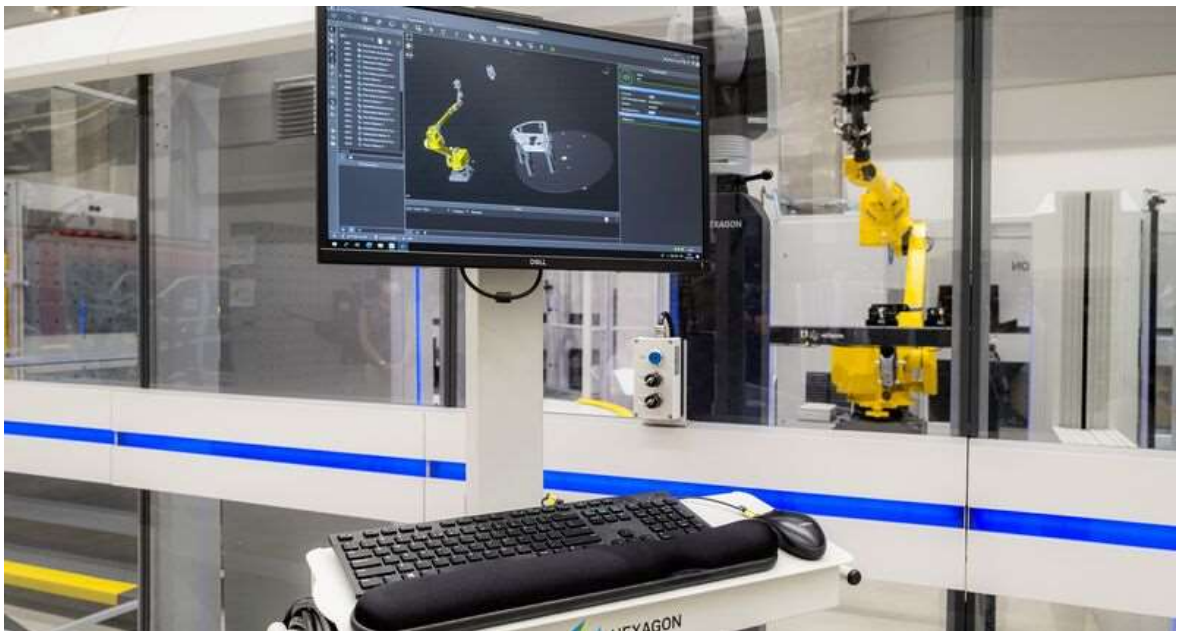
Figure 7. Industrial robot measuring system inside safety cage. The operating computer is placed outside of the parameter of the robot's working area. There is shutdown switch on the outside of the cage to turn the robot off for human intervention inside the working parameter. Without the safety systems there is a risk of serious injury or even death if human gets crushed or hit by the moving robot. [27]
