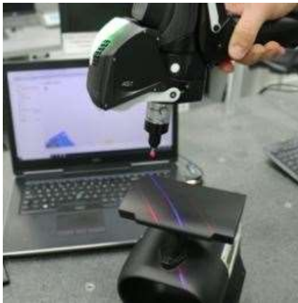
Figure 15. Absolute Arm 7-axis articulating arm wrist. Operator holds the device from the pistol grip and takes measurements using the red trigger. Scanner and probing head are both removable with repeatable mounting surface. The calibration certificate of the arm is valid for 12 months. [29]
