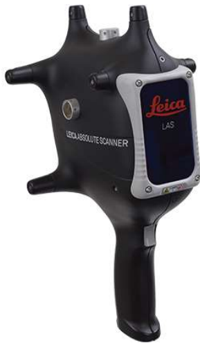
Figure 4. Handheld scanning device. The round objects on the end of the prongs are led lights that emit infra-red light. The larger cylindrical objects mounted on the sides, top and rear end of the scanner are reflectors that the laser tracker locks into. [18]
