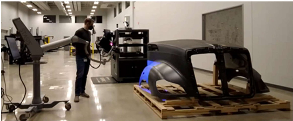
Figure 11. Plastic moulded truck engine cover panel inspected by photogrammetry device. With photogrammetry devices it is fast and easy to digitise the whole surface of a large-scale object. [33]
