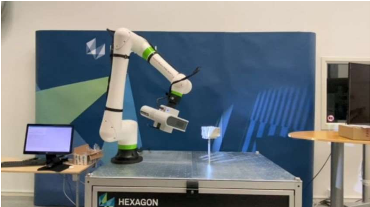
Figure 29. The first measuring position of the COBOT + Primescan system. The projected white light patterns can be seen on the demo part and at the wall behind the part.
