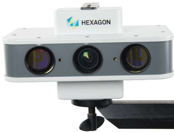
Figure 16. PrimeScan SLS scanner. It can be mounted to fixed stand or to moving object like robot. In the centre there is light projector and, on the sides, the angled cameras that catch the light pattern on the measured object surface. [30]
