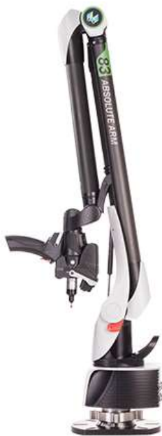
Figure 1. Modern articulating arm PCMM with 7-axes. Featuring contact probing head and laser scanner. User holds the device from the pistol grip and takes measurements using the trigger. In the base of the arm there is a handle to make it easier to carry the device around. [13]
