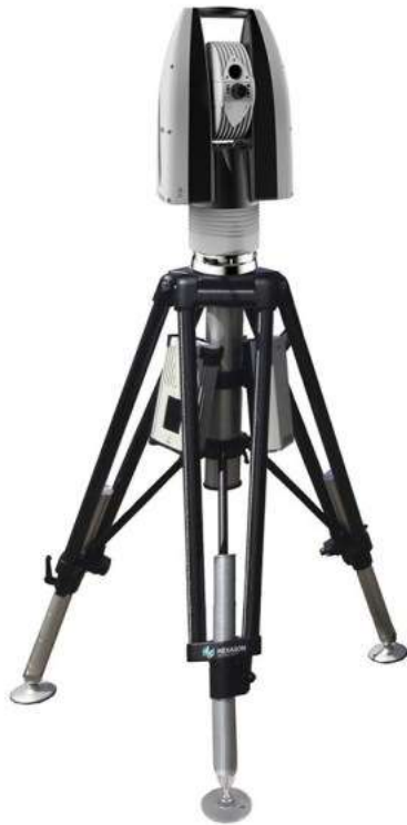
Figure 2. Modern laser tracker on a tripod. Attached to the centre pole of the tripod are controller for the tracker (left) and battery (right). Laser trackers can measure distances even up to 300 meters with few millimetres' accuracy. [17]
