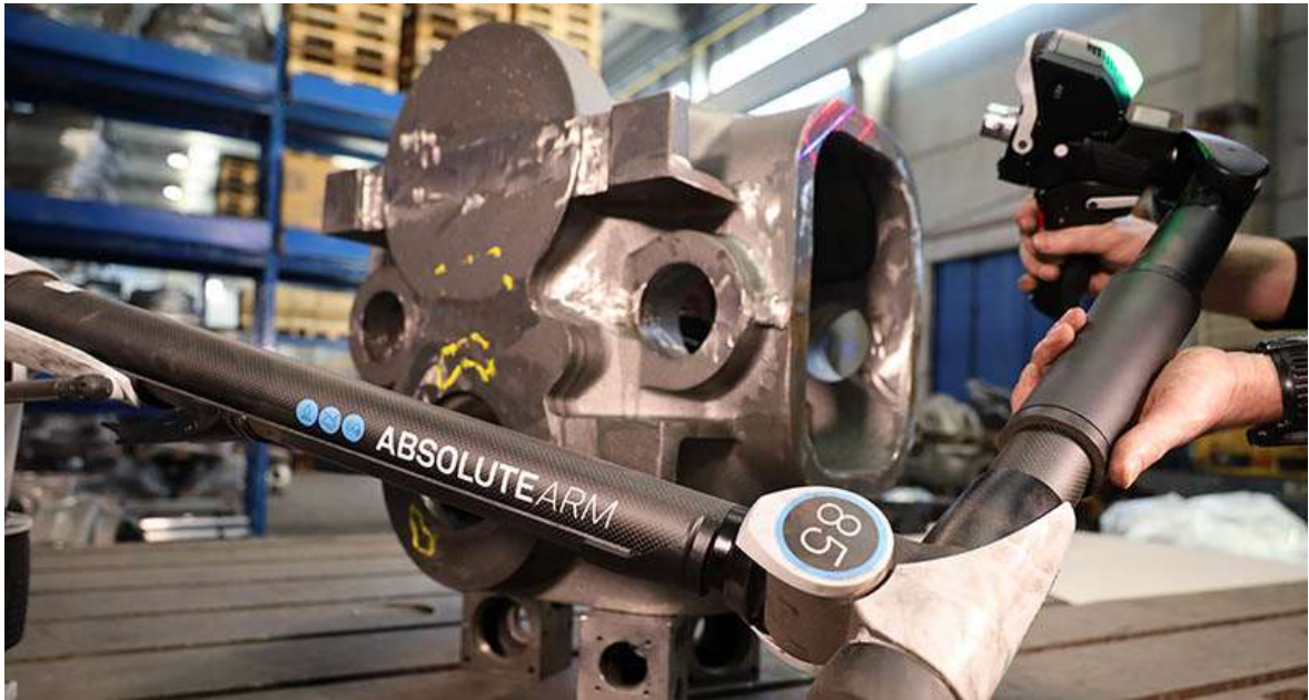
Figure 8. Articulating arm laser scanning metal part with complex shapes. [31]
