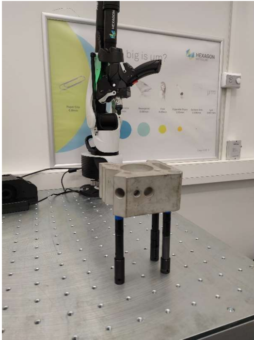
Figure 18. Premeasurement setup with the demo object suspended over three pegs. The articulating arm is fastened to the same threaded plate. The part was only held in place by gravity as laser scanning is contactless measurement type so there is no need to hold down the part during measurement. [25]
