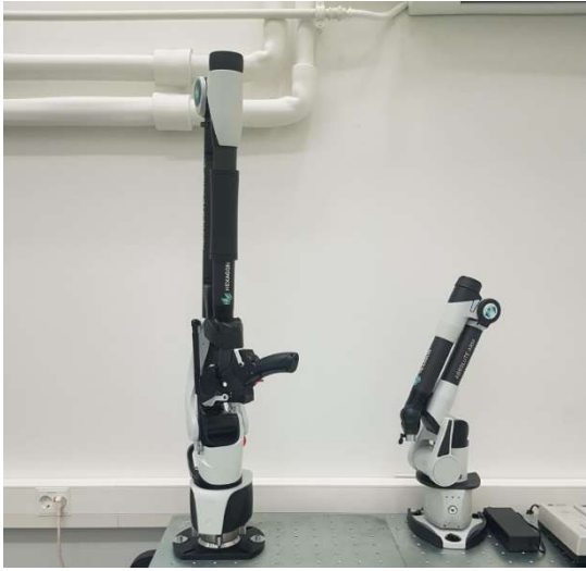
Figure 20. Compact Arm in the right and Absolute Arm 8525 in the left. The size difference between the two articulating arms is noticeable. Shorter shafts and fewer joints of the Compact Arm means higher measurement accuracy compared to the larger 8525 with longer shafts and extra joint, 7 axes versus 6 axes in the Compact Arm . [25]
