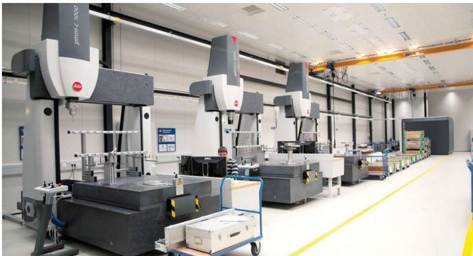
Figure 30. Modern CMMs in work. Modern CMMs are computer controlled. The operator is used to program the CMM trajectory and change the measured part when the CMM has finished measuring. [20]
