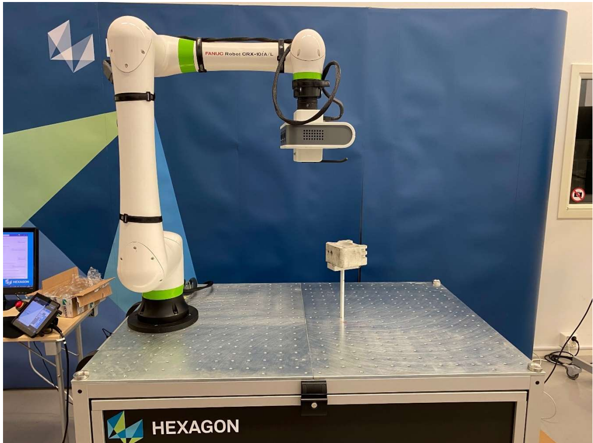
Figure 28. The COBOT + Primescan system measurement setup. A similar cart was used with the laser scanner setup also. The threaded tabletop is handy when setting up different kind of measurement situations.
