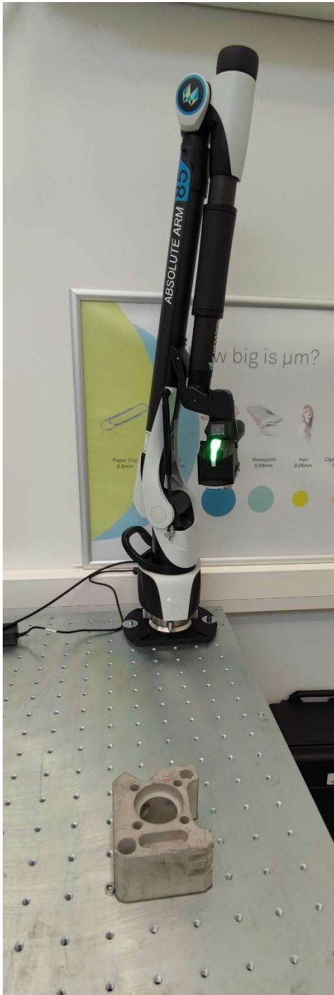
Figure 27. The positioning of the demo part in relation to the arm is like the premeasurement setup even though the support for demo part has been changed a little bit. The part is placed so that the laser scanner can reach all necessary surfaces of the demo part without the need to rotate the demo part. [25]
