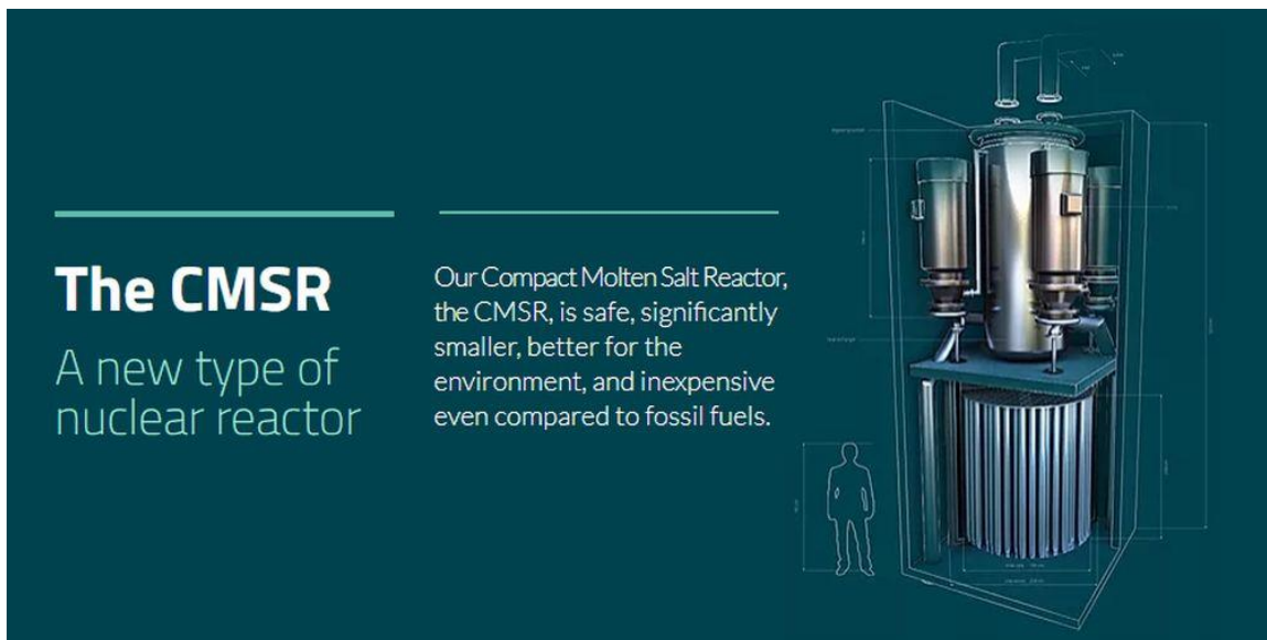
Figure 8. Seaborg CMSR design concept (Seaborg Technologies)
