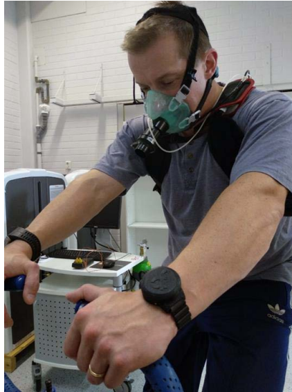
Figure 1.1. Subject from the project Q-Health wearing the first release prototype device equipped with HF and temperature sensors on his left hand. The device was used to measure EE from a wrist in a portable format with promising results when typical heart rate measurements were augmented with HF data (Levikari et al., 2020, Fig. 1.).
