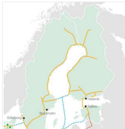
Figure 16. The Finnish hydrogen transmission network in the European Hydrogen Backbone. (Jaro et al. 2021, 23)
