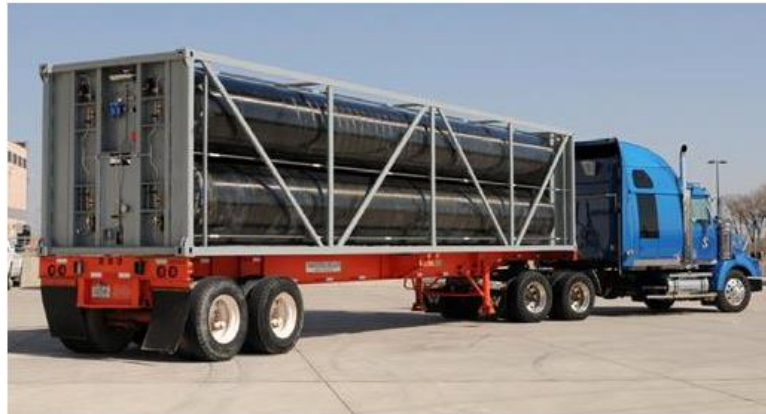
Figure 15. Titan CGH 2 tube trailer with 616 kg total hydrogen capacity at 250 bar. Pressure vessel outer diameter 1087 mm, length 11.67 m and weight 2175 kg. (Baldwin 2017, 9, 12)
