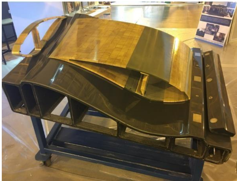
Figure 8: Blade mould and blade section by AM (Post et al., 2017)
