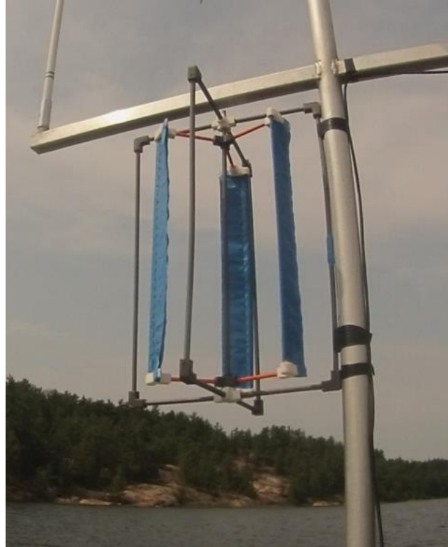
Figure 9: VAWT manufactured by AM (Bassett et al., 2015)
