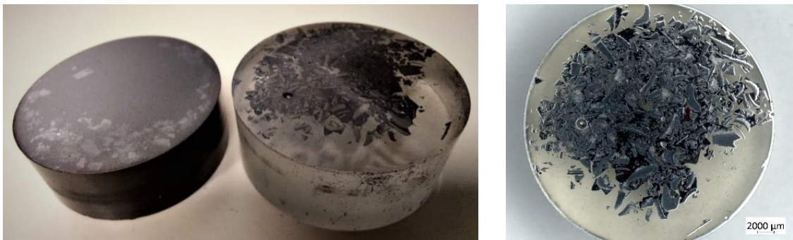
Figure 4.7. Magnetite powder from the Loviisa NPP cast in conductive SEM resin (left) and epoxy resin (right).
