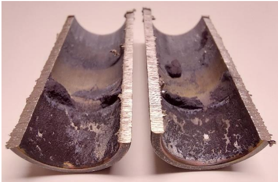
Figure 5.8. Deposited and hardened magnetite from the 8 th pipe cell experiment.
