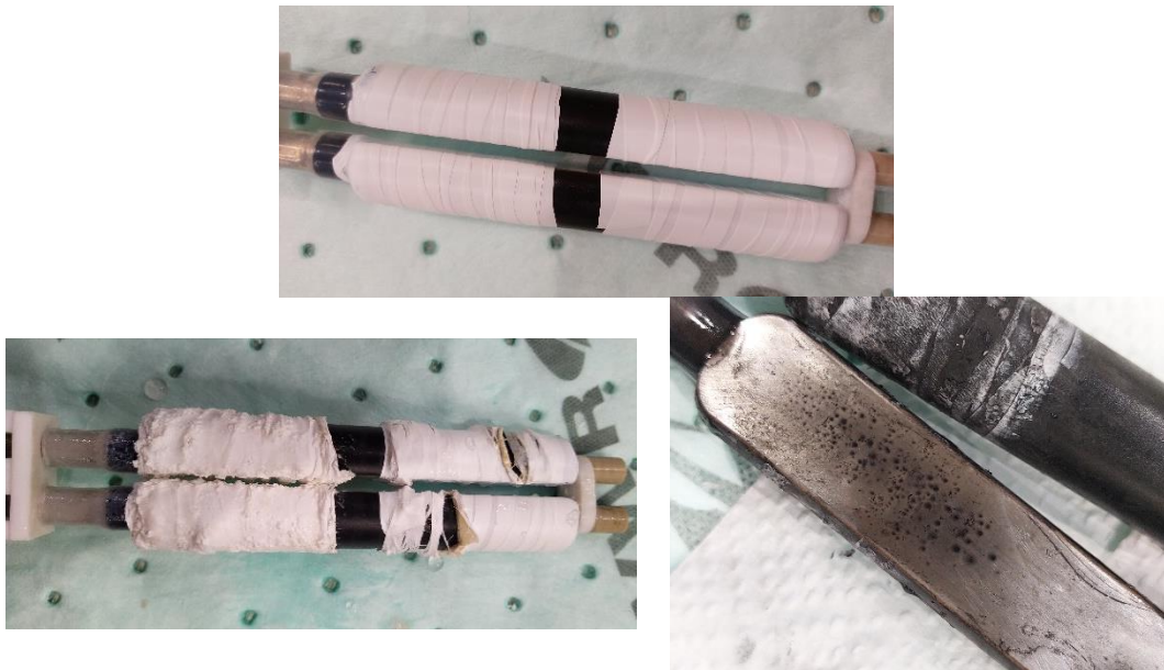
Figure 5.11. Metal blocks lined with Teflon tape to reduce surface area (up) and pitting corrosion on the metal surface as a result of heavy boiling between the tape and the metal surface (down).
