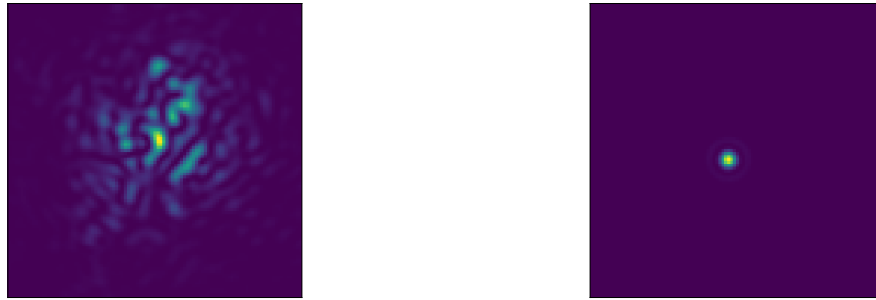
(a) Uncorrected image with visible speckles.
