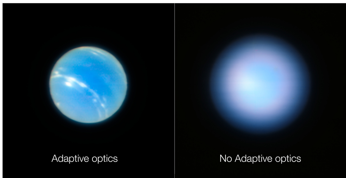
Figure 1. Neptune imaged using Very Large Telescope with and without AO [1].
