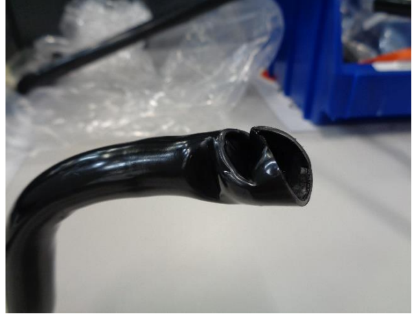
Figure 3 Production error due to machine defect
