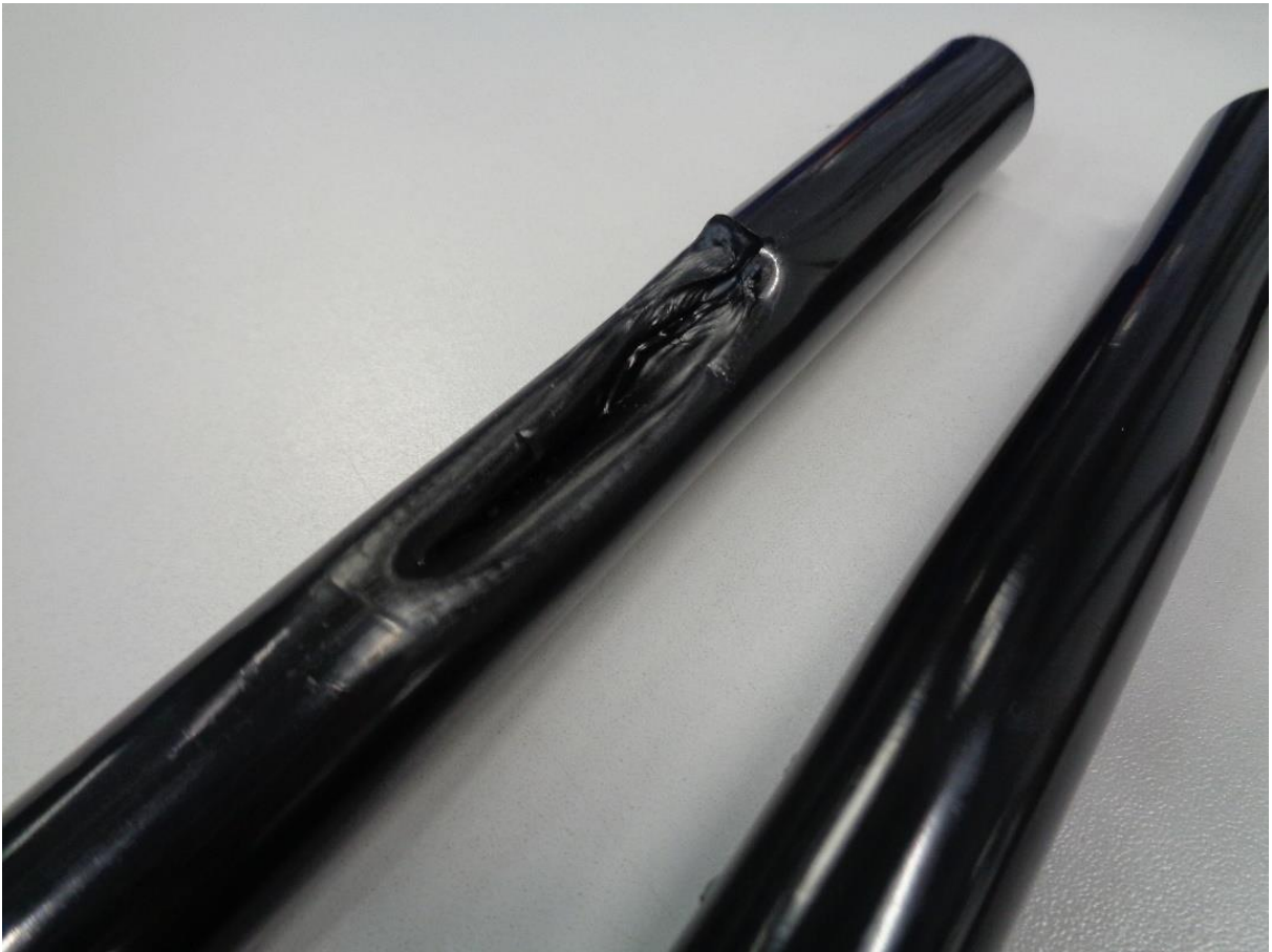
Figure 4 Production error due to worker inattention
