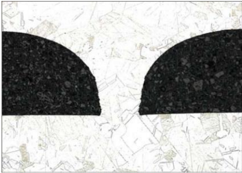
Figure 41 Grain pattern at a diffusion bonded joint (Heatric, 2018)
