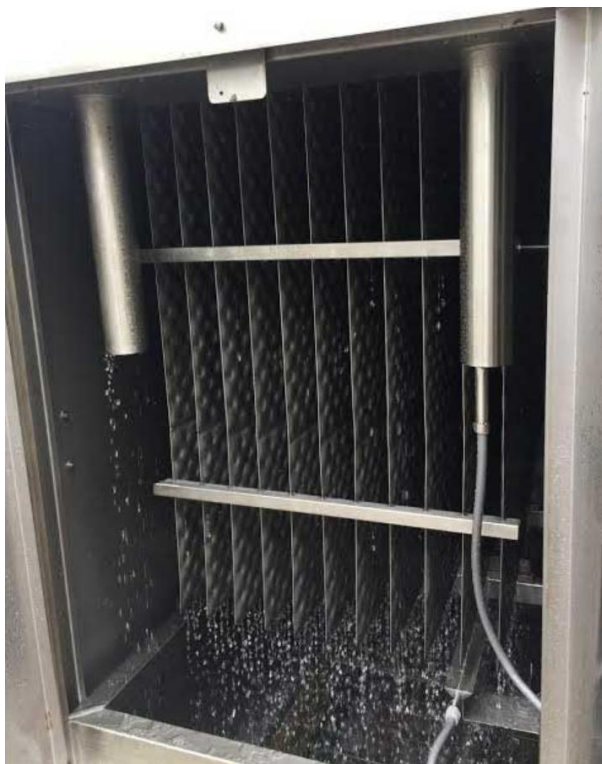
Figure 39 Falling film evaporator (Omt-triaca, 2022)
