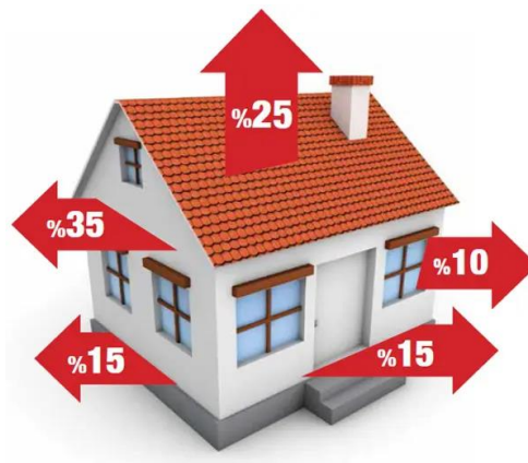
Figure 4.1. Heat loss in single-family house (Dmytro et al., 2017): Walls (35%), Roof (25%), Floor (15%), Infiltration through windows and doors (25%)
