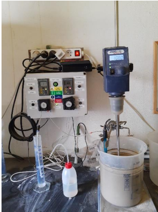
Figure 29. Leaching process with CNLite with automatic NaOH control
