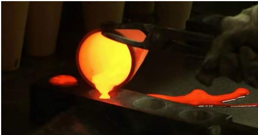
Figure 15. Ceramic crucible with melted sample (Jenkin et al., 2016, 18–24)
