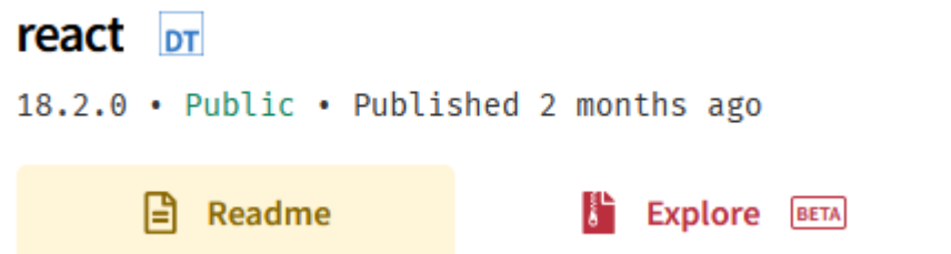
Figure 10. A npm package that has a DT icon next to its name, which means that it has a separate type package under Definitely Typed.
