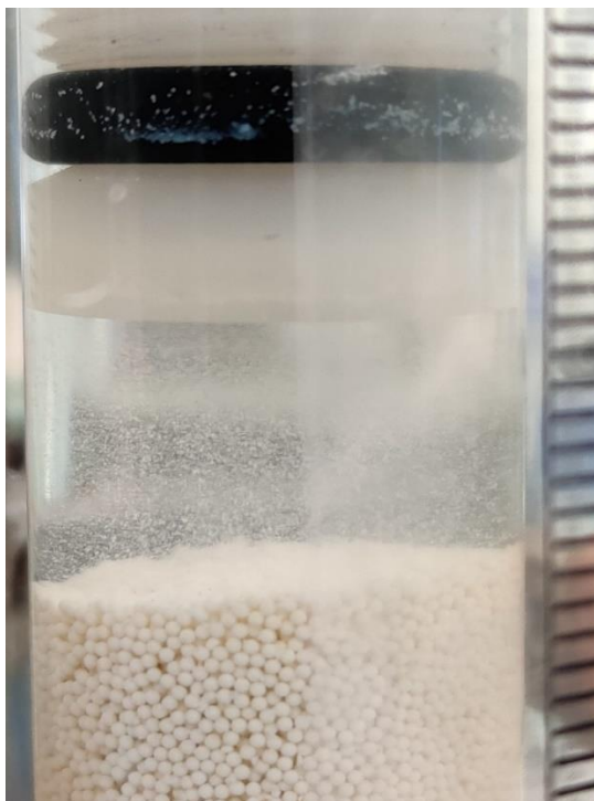
Figure 16 Precipitation inside ion exchange column after elution of Al.
