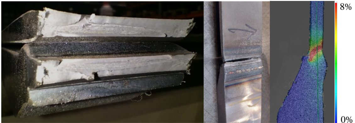
Figure 31. The ductile fracture at 96G26_S1 specimen. Failure happened in the softened HAZ at S960 plate. Necking and a high strain line can be detected in HAZ where failure happened.
