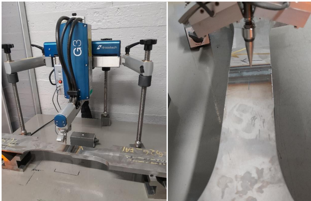
Figure 24. X-Ray diffractometer setup on residual stress measurements.
