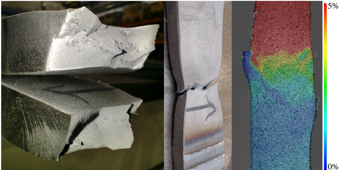
Figure 28. The ductile fracture at 35G26_S1 specimen. Failure happened at S355 base material outside DIC capturing area and no high strain regions can be detected in weld area from DIC image.
