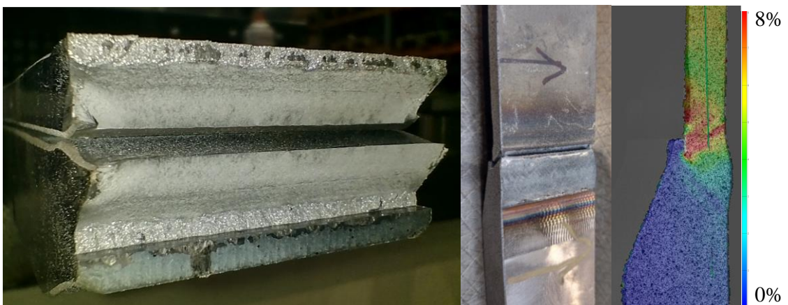
Figure 30. The brittle fracture at 70G26_S1 specimen. Failure happened on S700 HAZ and one high strain line can be detected in failure location.
