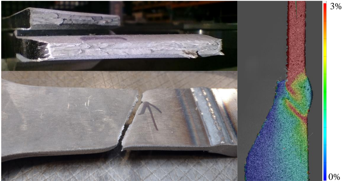
Figure 32. The ductile fracture at 11G26_S1 specimen. Failure happened at S1100 base material outside DIC capturing area. In DIC image two higher stain regions can be detected, one from the weld root, possibly following the fusion line and other on cast steel HAZ.
