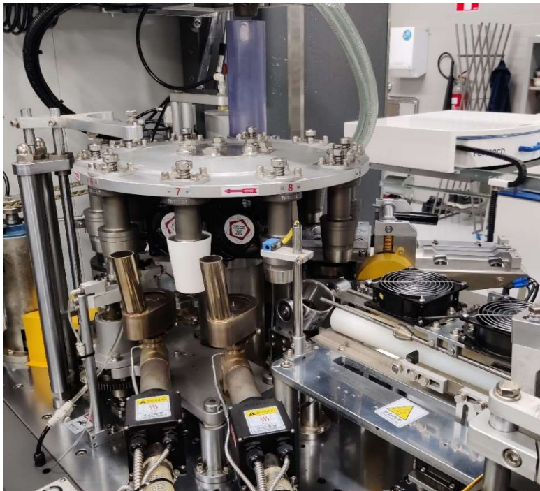
Figure 10. Cup travelling in a mold perpendicular to the horizontal revolver, situated between the bottom heaters. The side seams are cooled by fans before entering the bottom forming steps.
