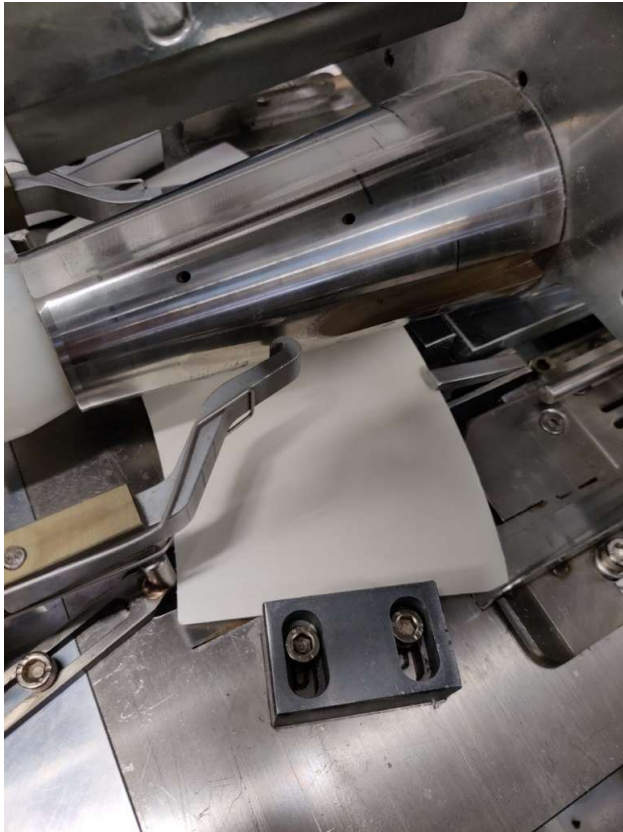
Figure 12. Blank positioning tools used for side seam sealing.
