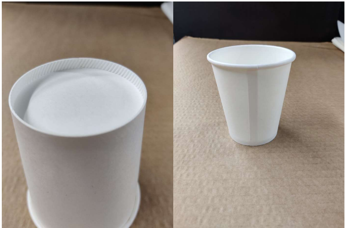
Figure 20. A cup formed from experimental material 3. The dimensions are within the set tolerances and the cup has no visible defects
