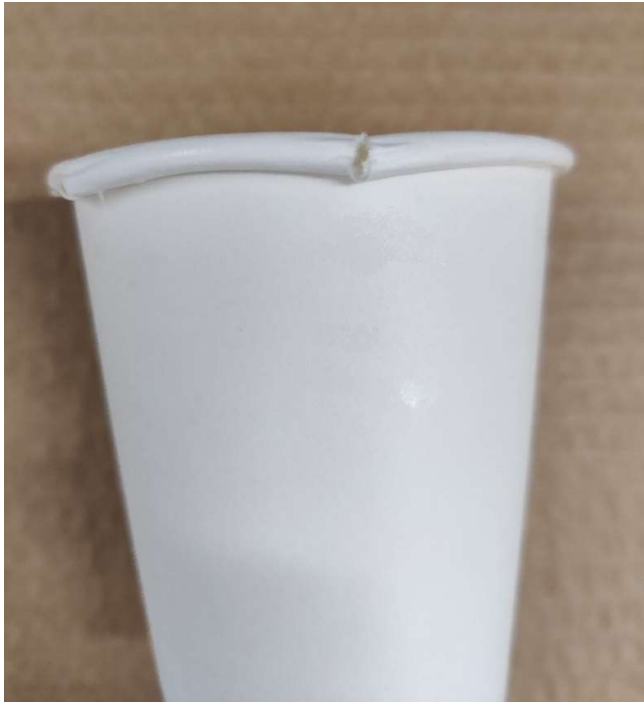
Figure 28. Split rim roll caused by dry cupstock. 2-side biopolymer coated paperboard
