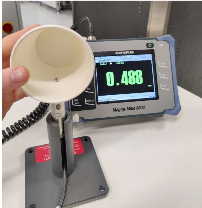
Figure 43. Measuring the thickness of the side seam at the middle point
