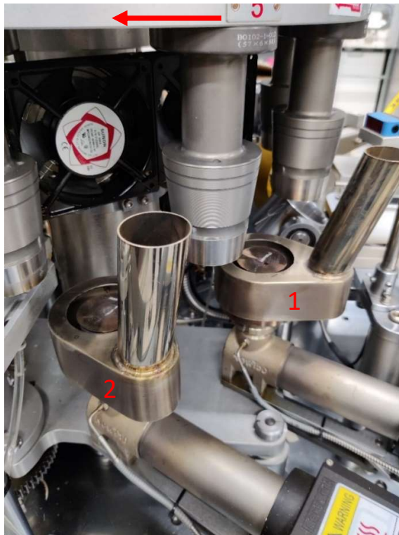
Figure 13. Bottom heating stations. The direction of rotation is marked with a red arrow.
