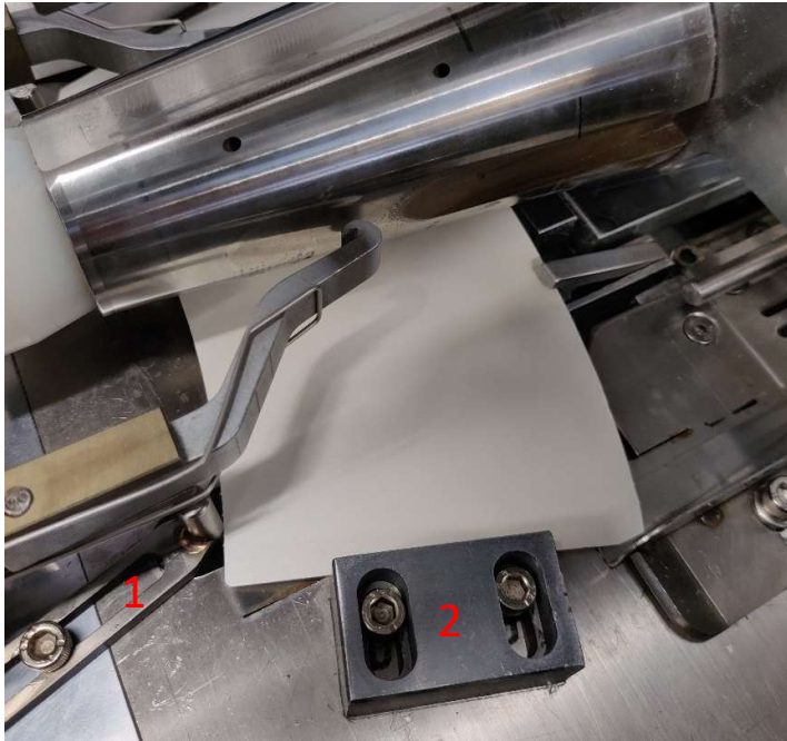
Figure 29. Original positioning system. The stopper peg (1) and guide piece (2) have identical counterparts on the other side of the mandrel, not visible in the figure.
