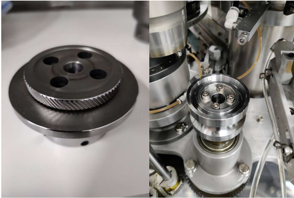
Figure 3. Left: Patterned knurling tool. Right: Curling station (LUT packaging laboratory)
