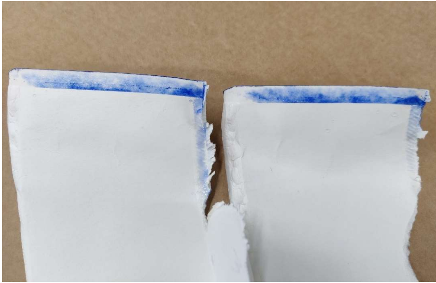
Figure 37. Torn side seams of cold run (left) and hot run (right) with added dyed soap water displaying the portion of fiber tear.
