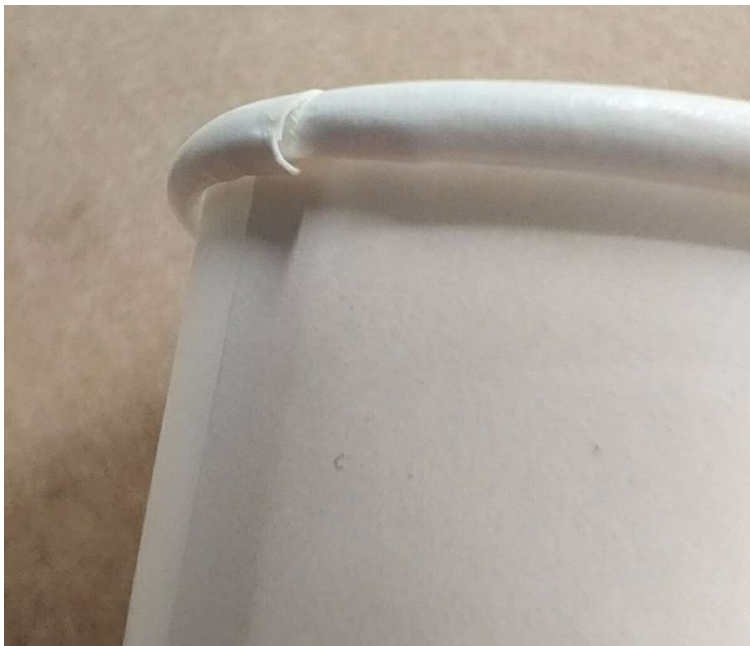
Figure 25. Opened rim roll caused by incomplete side seam. Two-side dispersion coated paperboard
