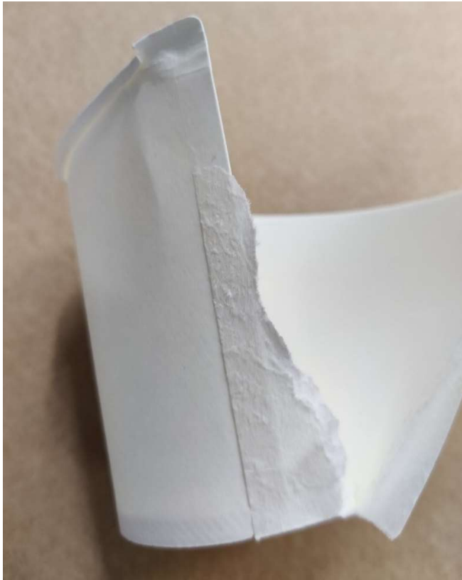
Figure 24. Incomplete side seam, two-side dispersion coated paperboard.
