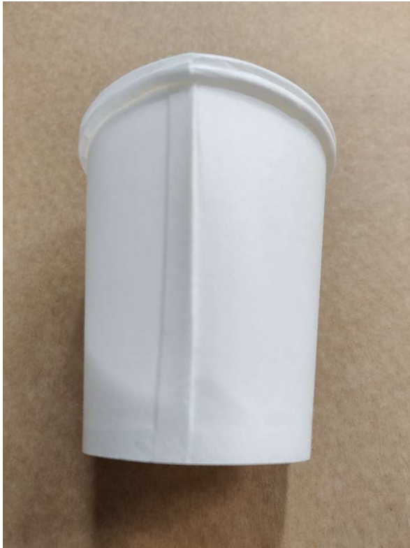
Figure 27. Folded side seam and rim roll on a defective cup
