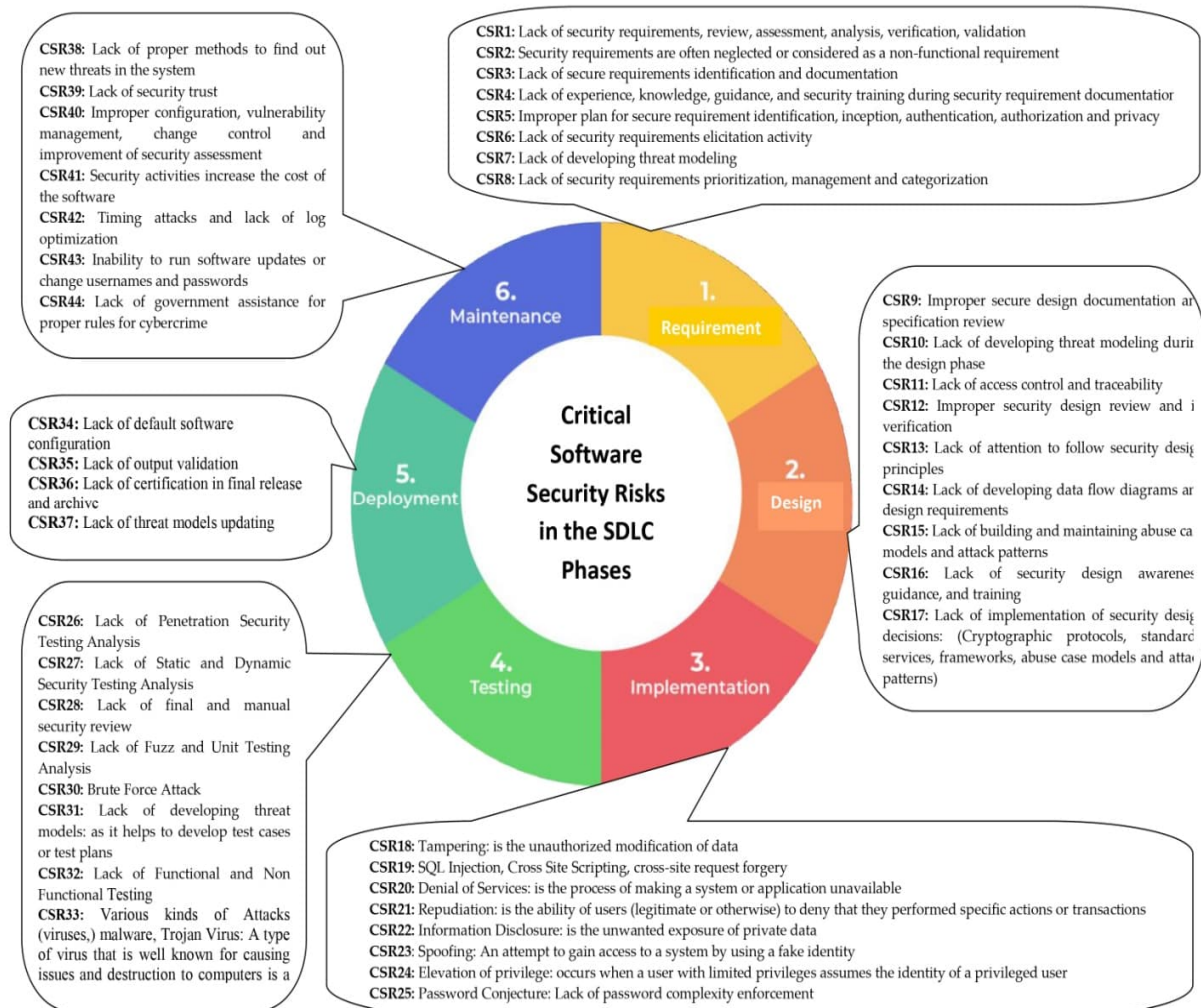
Figure 6: Theoretical model of the critical software security risks of SDLC in GSD
