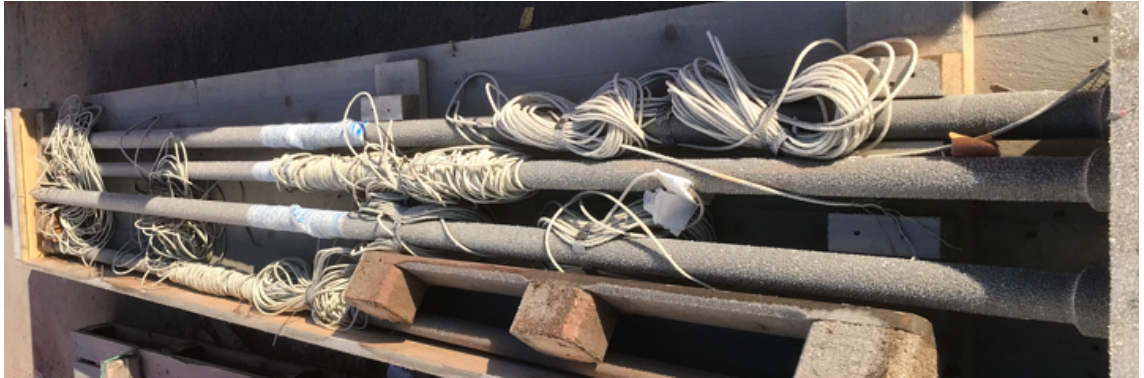
Figure 9. Strain gauge rods with strain gauges installed.
