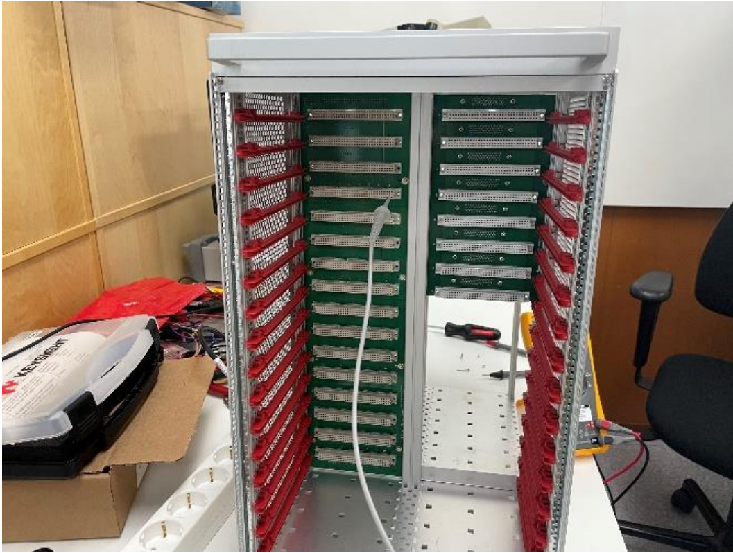
Figure 16. Oscilloscope probe attached directly to a connector slot.
