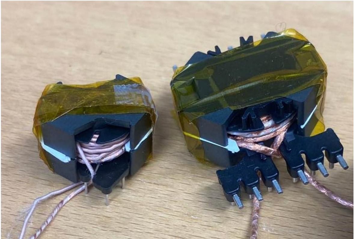
Figure 51 Built RM 7 (left) and RM 10 (LP) cores.
