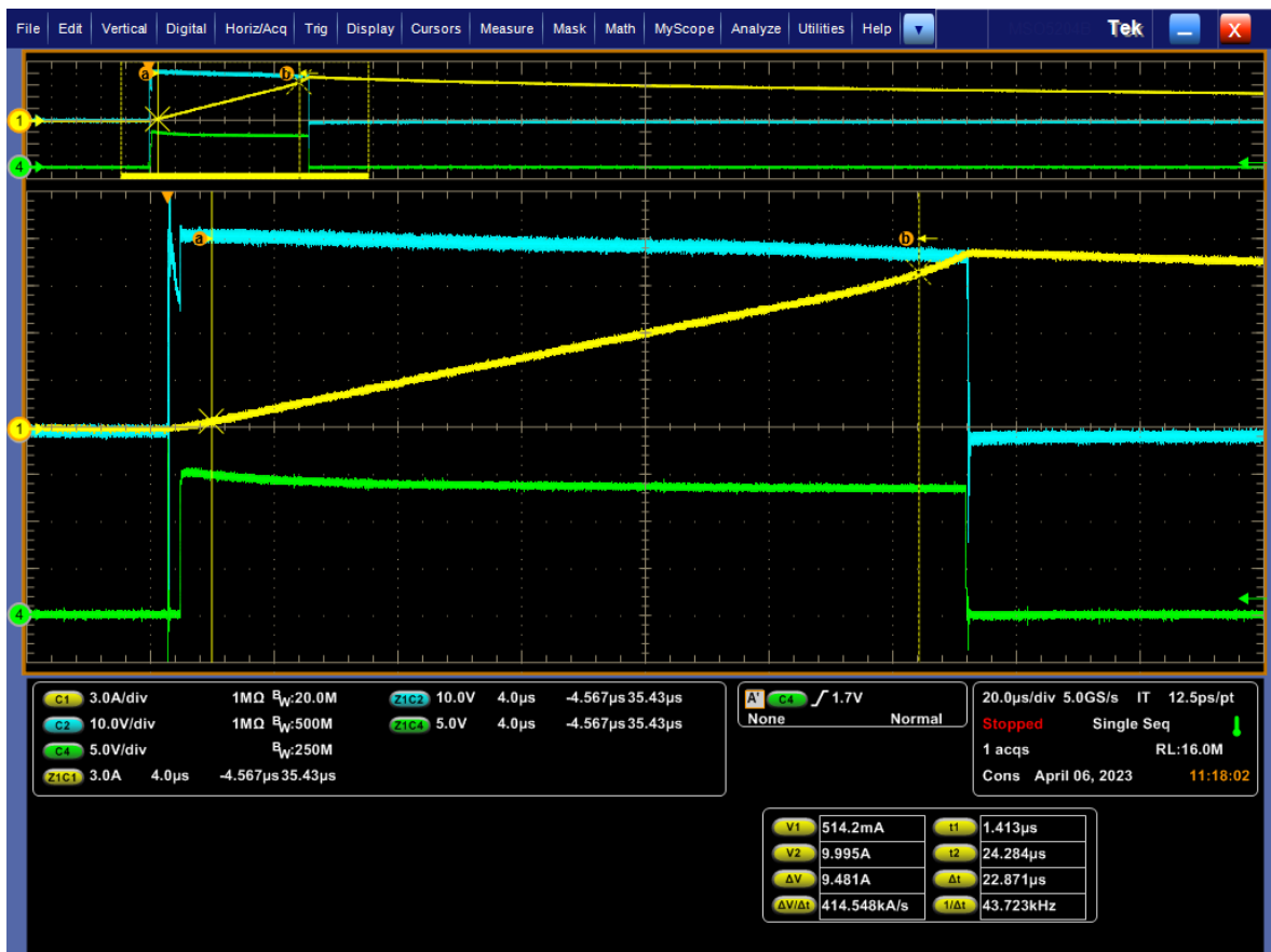
Figure 62 Single-pulse test of the choke with targeted 80 \mu H.
