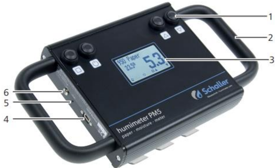
Figure 12. Picture of the Humimeter PM5 paper moisture meter. 1. Selection button, 2. Handle, 3. Display, 4. USB port, 5. Reset button, 6. LED battery indicator (Schaller Messtechnik GmbH 2022)
