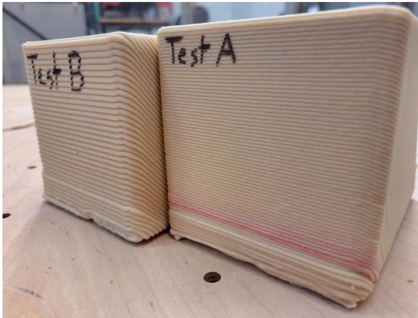
Figure 21. Test print of a boxes with 1 and 2 mm layer heights in 45-degree angle with 6 mm nozzle and 10 mm layer width
