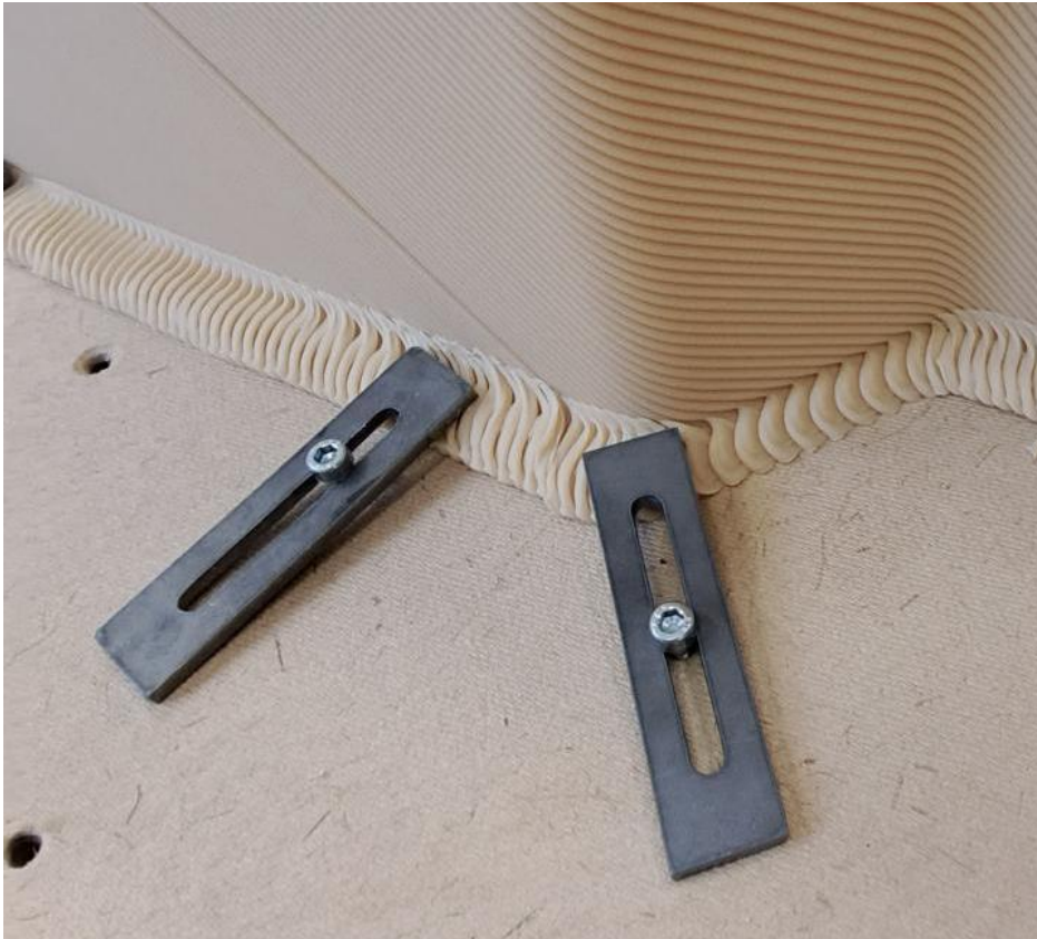
Figure 29. The integrated raft to be used of clamping of the printed part on the bed
