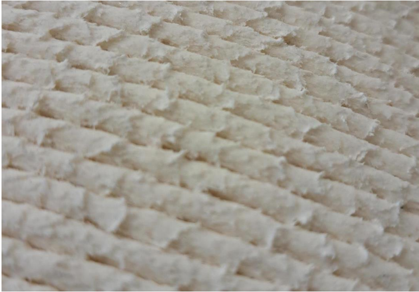
Figure 31. Cracks in beads due to under extrusion caused by material dragging with nozzle
