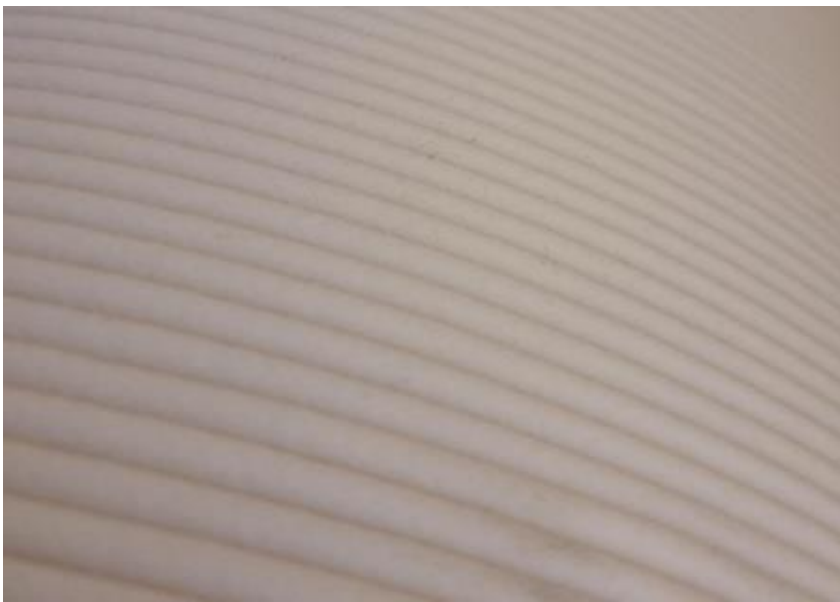
Figure 32. Acceptable surface quality with increasing the flow ratio and bead width
