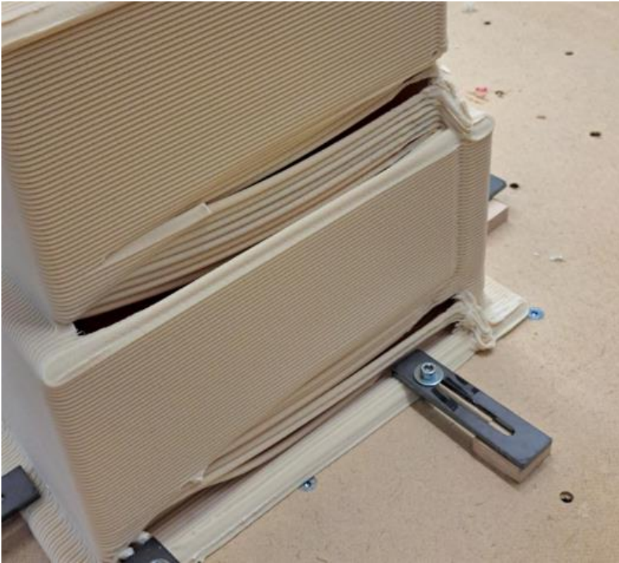
Figure 24. An example of failure due to long bridging in angled sliced print
