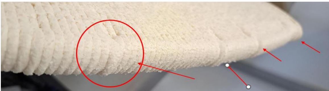
Figure 42. Buffer lag in movement of robot causing print quality failure
