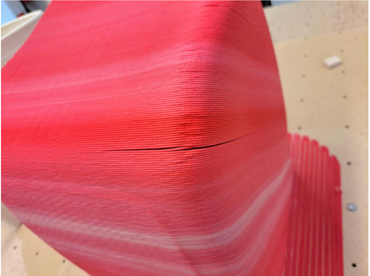
Figure 41. The occurrence of cracks during the printing process was attributed to thermal stresses and inadequate bonding between the layers
