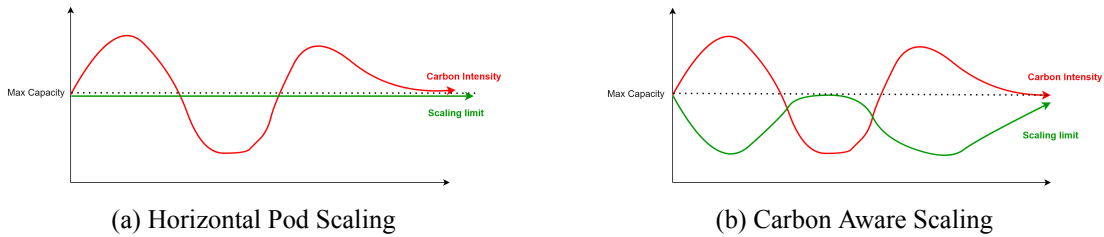
Figure 3: visualization of how the scaling capacity of software changes for both Horizontal Pod scaling and Carbon Aware Scaling
