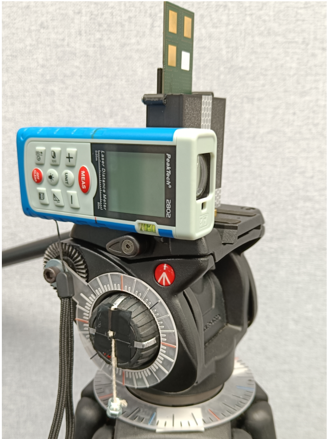
Figure 18: Protractor discs were 3D printed for easier adjustment of the azimuth/elevation angles. A laser distance meter was mounted to the side of the main DUT enclosure.
