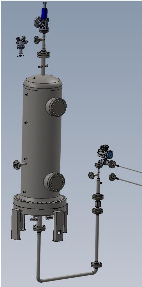
Figure 34: C-FLOW test facility main components (C-FLOW test facility 3D model revision v.1).
