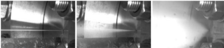
Figure 26: Examples for specific flow patterns: Jet only (left), jet and steam cone (center) and steam cone only (right) (Heckmann et al., 2022).
