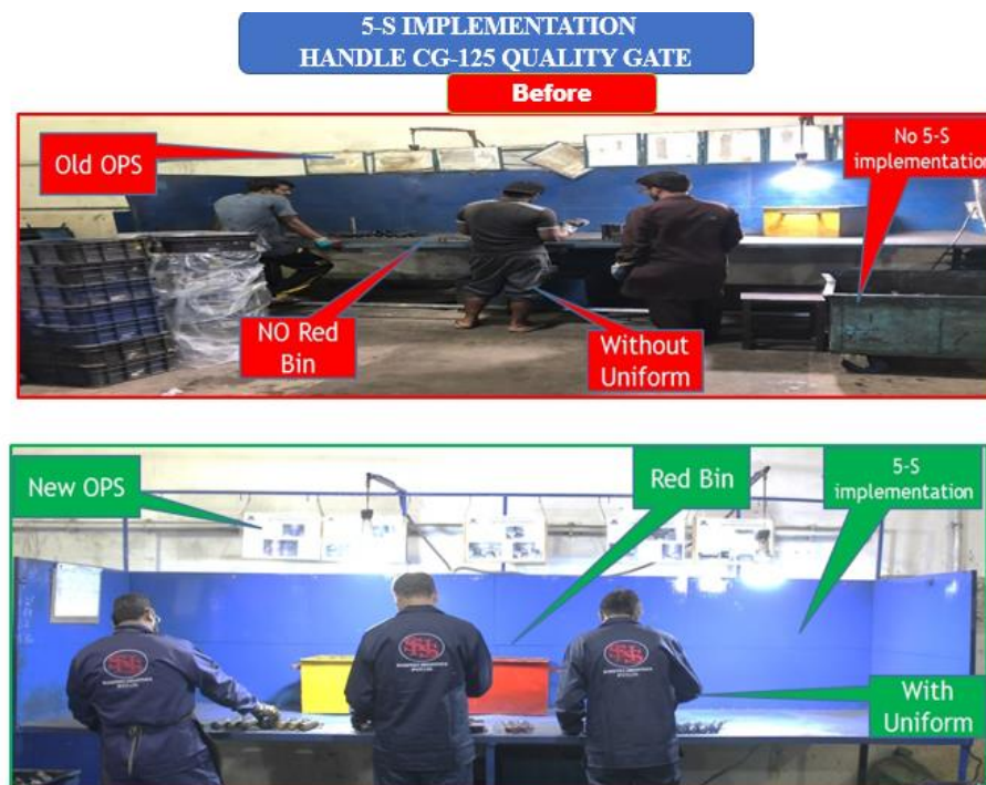
Figure 20. 5S Implementation at Handle CG-125 Final Inspection Quality Gate
