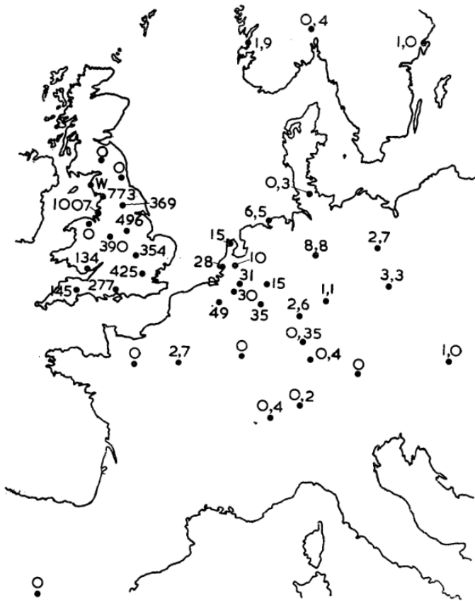
Figure 5. A map displaying the time integral of the concentration of ^{131}\text{I} in the air (micro-microcurie-days per cubic metre) in Europe following the Windscale accident in October, 1957 (Loutit et al. 1960).
