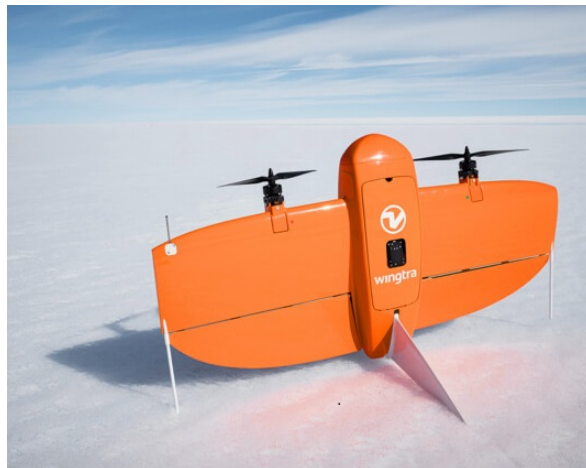
Figure 10: Example of a Tail-sitter VTOL UAV type ( Tailsitter VTOL | PX4 User Guide (main) 2024 )
