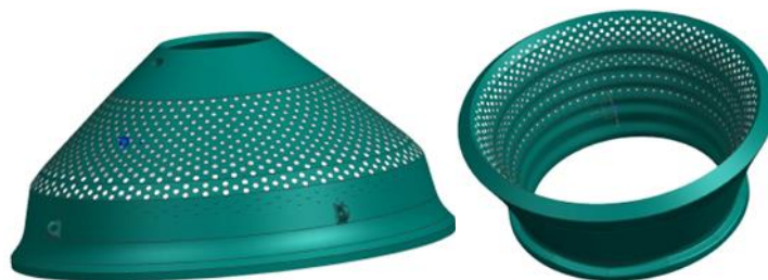
Figure 1. Mantle and bowl liner for HP cone crusher machine
