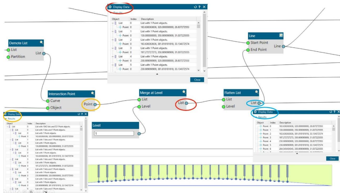
Figure 24. Creating a line from the insert surface points to the back surface points
