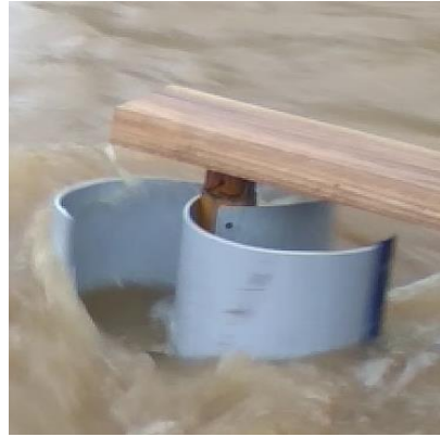
Figure 6. Savonius water turbine in operation (Zafar, 2018)
