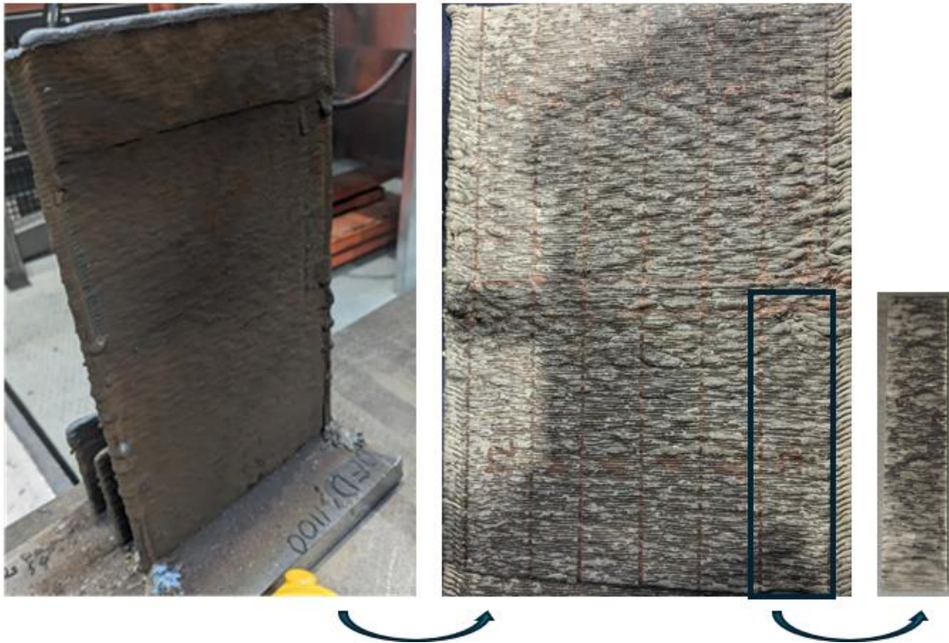
Figure 4: Presents the preparation of test specimens from WAAM plate.
