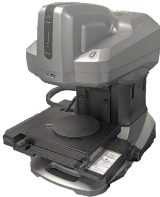
Figure 5: Presents the 3D profilometer which was used to scan the test specimens.
