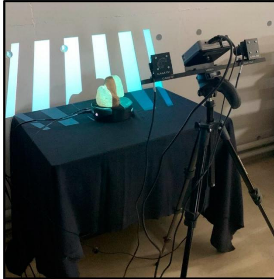
Figure 4. Scanning of fossil coral colonies with Scan-in-a-box structured-light scanner.
