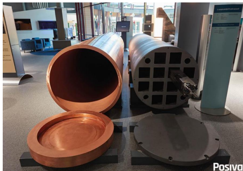
Figure 3.3 Copper overpack and cast-iron insert (Posiva, 2024g)
