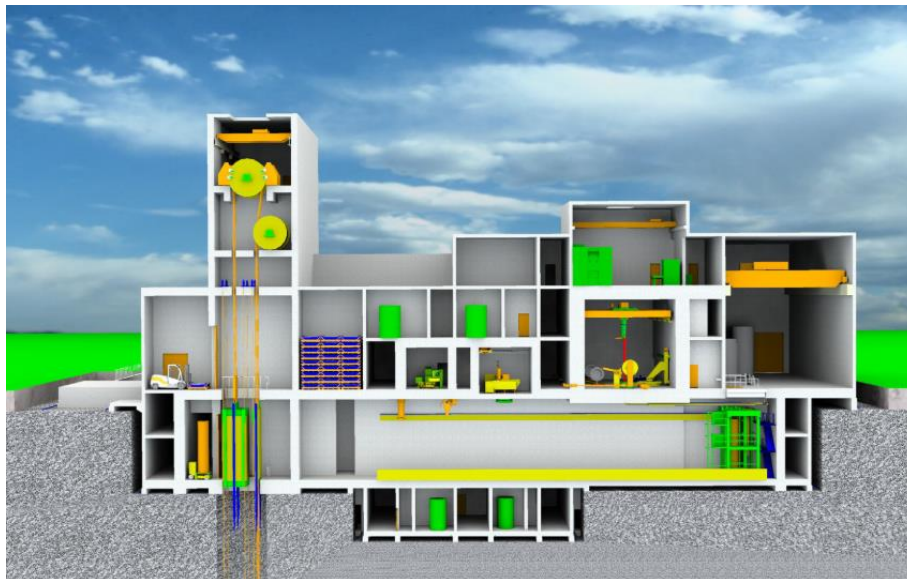
Figure 4.2 Longitudinal section of the encapsulation plant (Kukkola, 2012)
