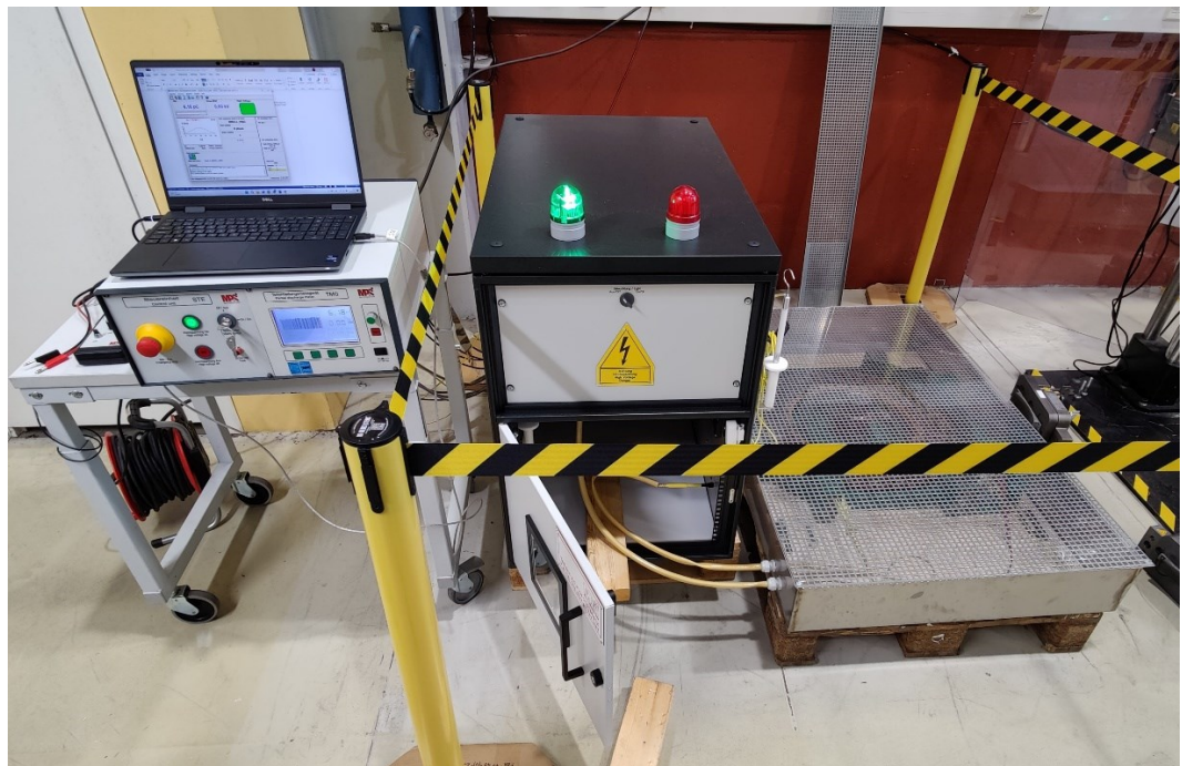
Figure 12. The test setup for measuring the partial discharges.
