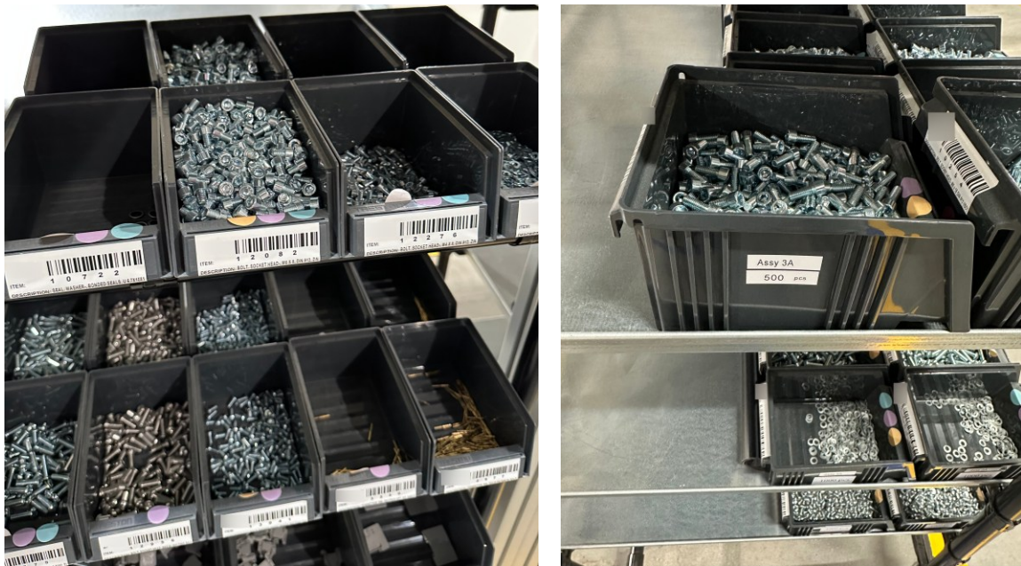
Picture 10. Labelling on the line-side stocked small pieces.
