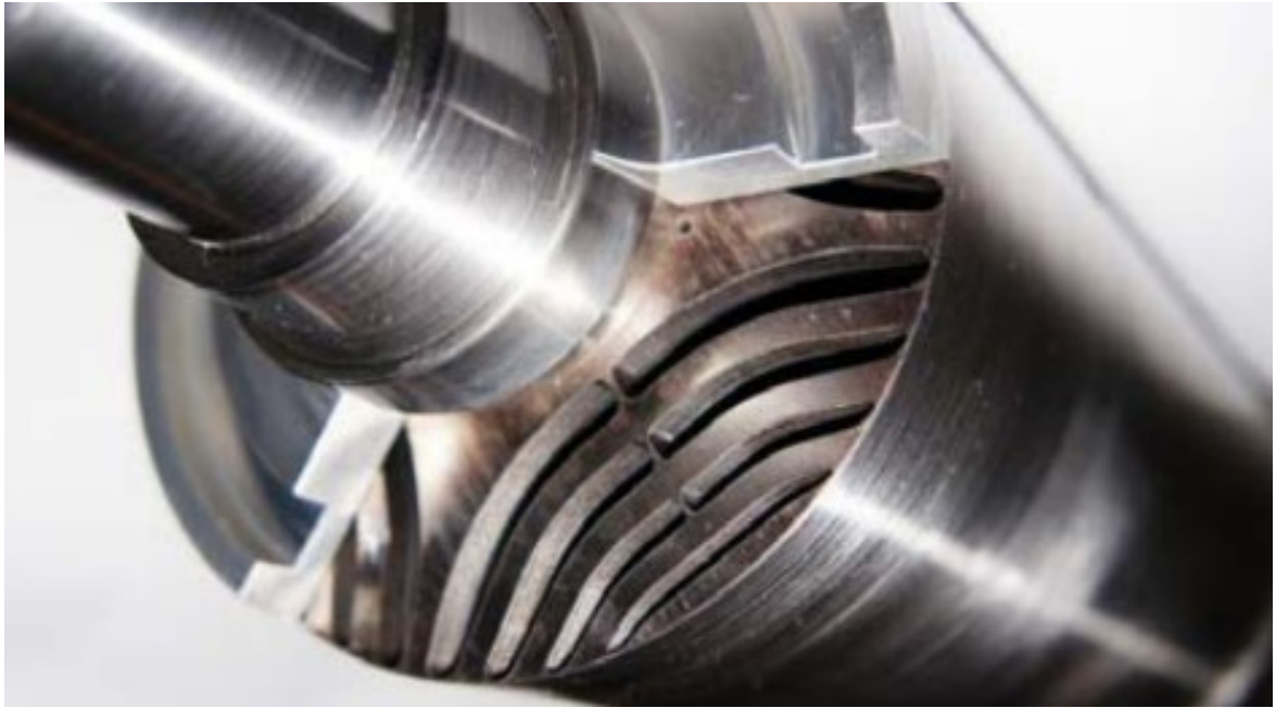
Figure 2. structure of Rotor in SynRMs (Taghavi & Pillay, 2014, p. 330).
