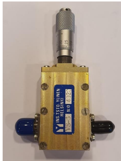
Figure 1. The photo of the discussed phase shifter
