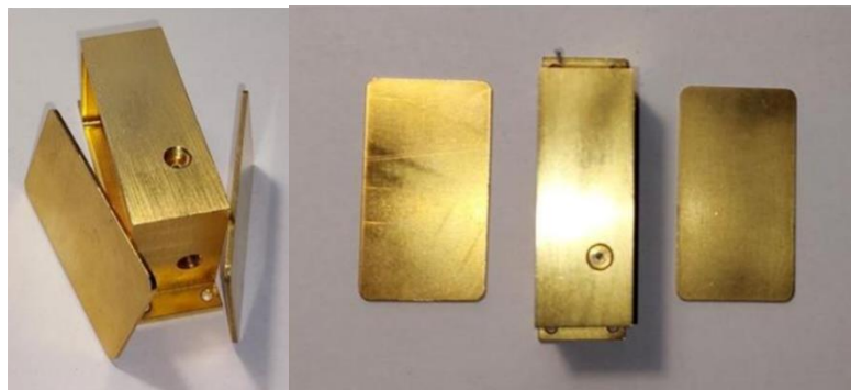
Figure 1: Ultra-low noise microwave amplifier for planetary space probes.
