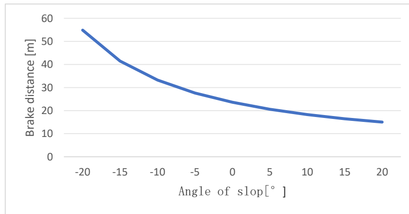
Figure 11. Comparison of slope Angle and braking distance.
