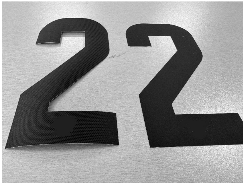
Figure 15. On the left, cut Twill fabric/Adhesive 02 presenting slight curl, on the right (flat) control product.
