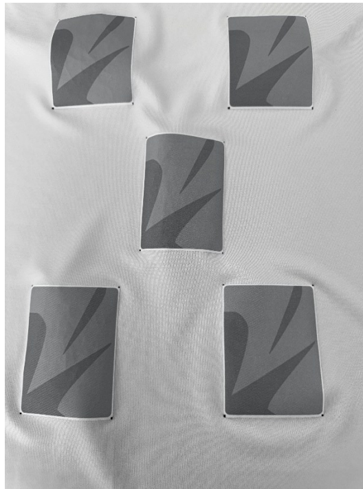
Figure 16. Twill/Ind trial samples after 5x 60degC wash and tumble dry cycles. Tumble dried samples present curling.
