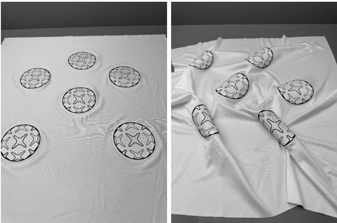
Figure 17. Standard product (on the left) and Twill/Ind trial samples after 10x 60degC wash and tumble dry cycles. Twill/Ind trial samples present extensive curling after conditioning.
