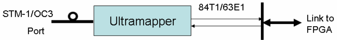
Figure 28 Main function of Agere Ultramapper is to transmit E1/T1's from fibre to FPGA
