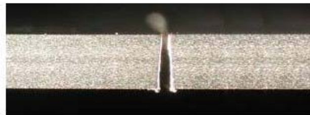
(c) A wider kerf width at the bottom
