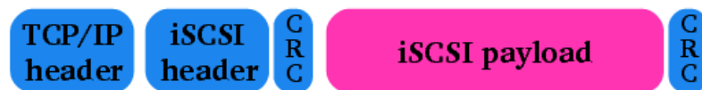
Figure 7: Packet fields in iSCSI protocol, with partition-level encryption applied to payload. Purple indicates encrypted content.
