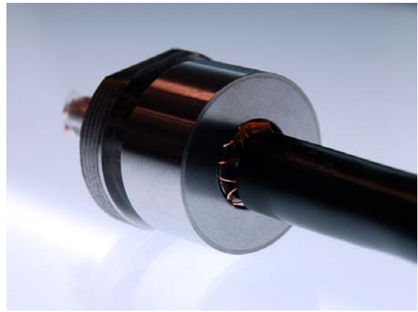
Figure 7.4. The feeder cable is fitted in the gland. The phase conductors are threaded through the gland and the grounding conductor is fitted between the conical part of the gland and the lock ring. The outer covering, which tightens the connection, along with the possible standard cable gland is not shown.
