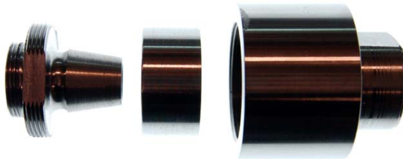
Figure 7.5. The prototype including the gland, the lock ring, and the outer covering. The standard cable gland used to secure to cable is not shown.
