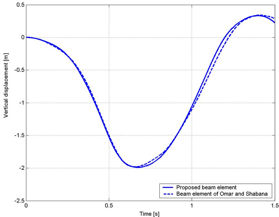
**Figure 9. A comparison of the vertical displacement between the proposed element and that presented by Omar and Shabana using 4 elements.**
